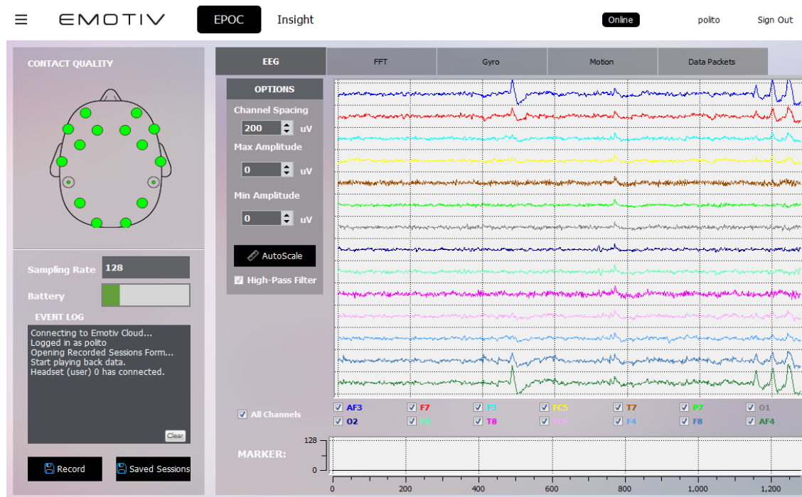
Figure 12 – EMOTIV XAVIER Pure EEG real time display
