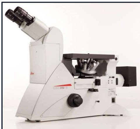
Figure 7.2 – The inverted optical microscope used for 3D-printed piezoelectric scaffold imaging.
