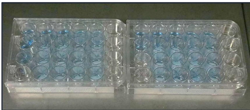
Figure 6.12 – AlamarBlue was added to each well with a 1:11 ratio.
