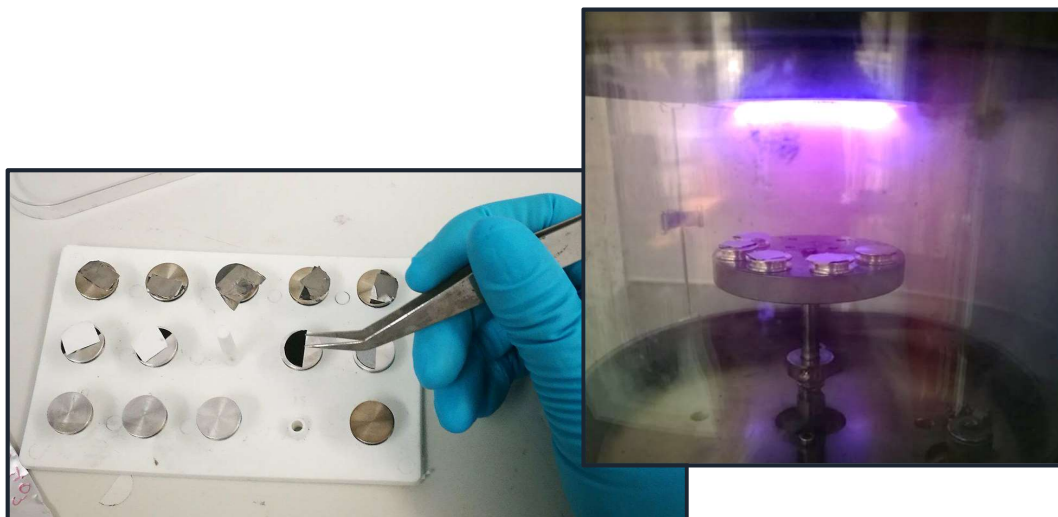
Figure 6.1 – The samples were prepared to be gold sputtered by using an argon plasma.
