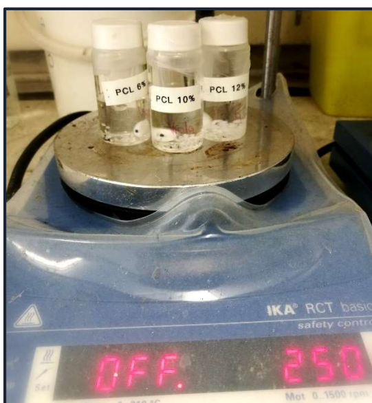
Figure 4.3 – Solutions of PCL and DCM were mixed under magnetic stirring (250 rpm) at room temperature overnight.
