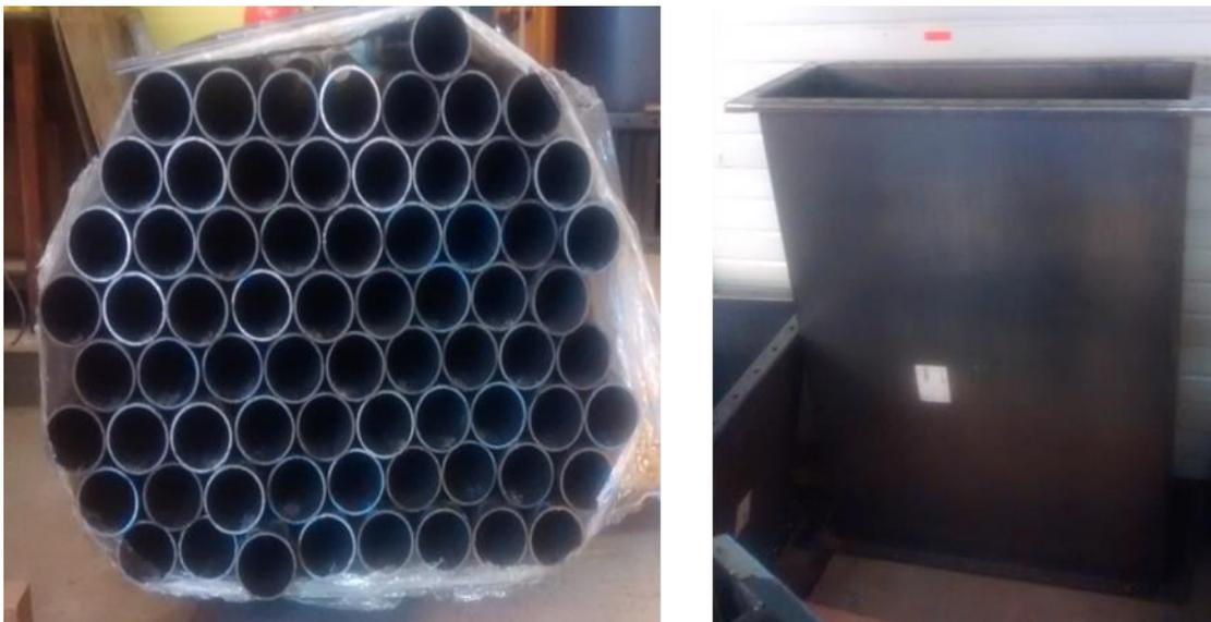
*Figure 41. Tubes and duct used for the flow straightener construction.*
