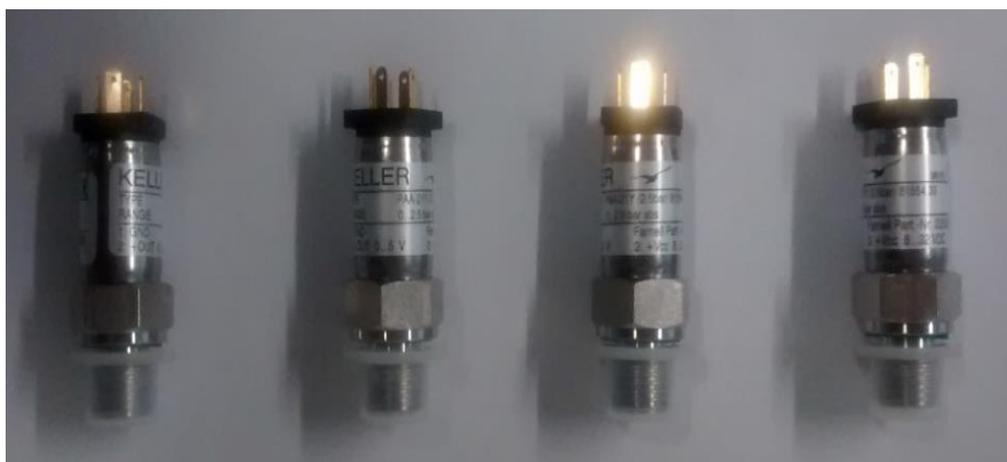
*Figure 54. Picture of the absolute pressure sensors.*
