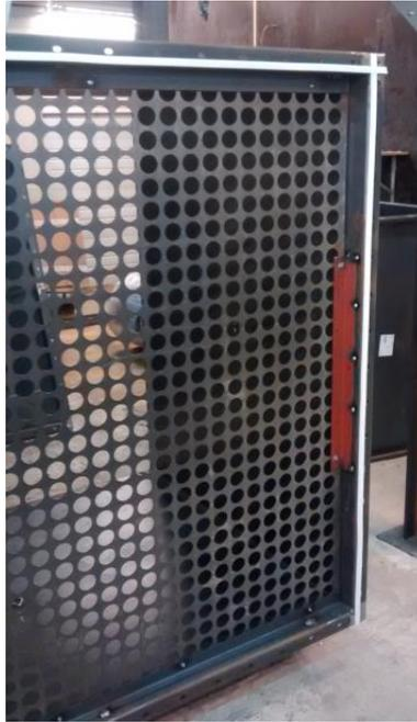
*Figure 52. Picture of the perforated plate used as settling mean.*
