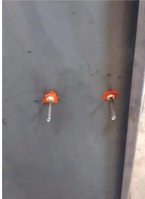
*Figure 53. Picture of the pressure taps installed.*
