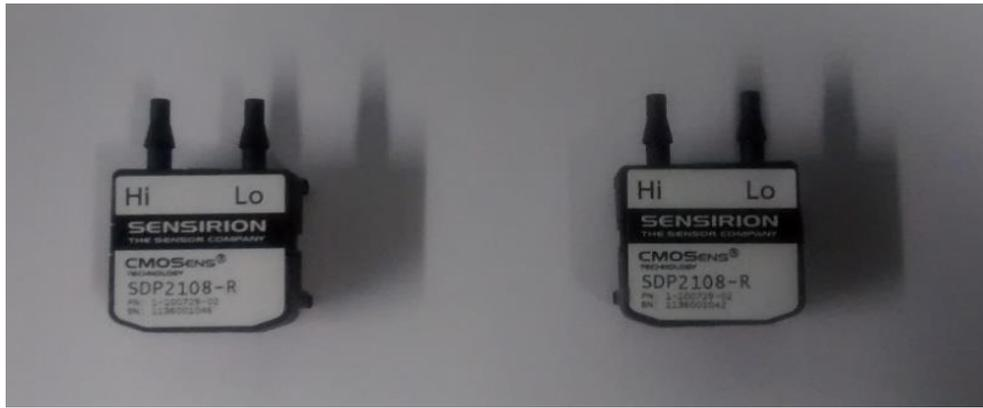
*Figure 55. Picture of the differential pressure sensors.*
