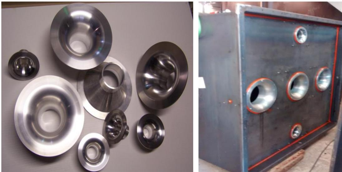
*Figure 51. Images of the metallic nozzles used and the nozzles attached to the perforated fixation plate.*
