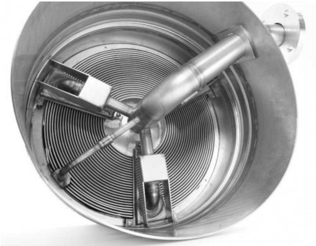
*Figure 28. Picture of one side of the GAP 50-3-3 heat exchanger [19].*
