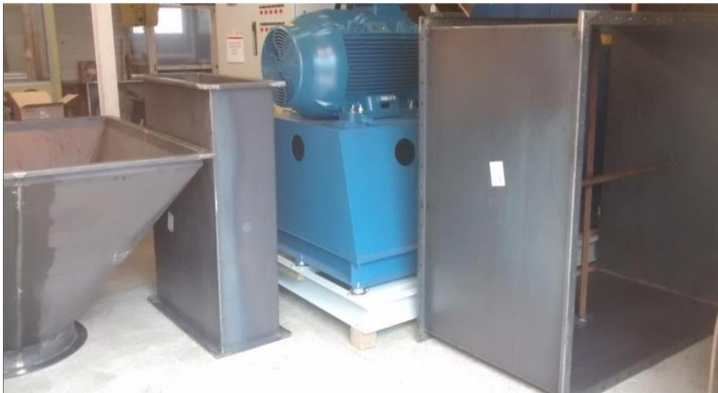
Figure 46. Picture of various ducts used for the test bench construction.
