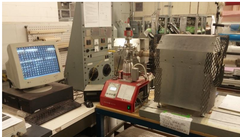
Fig 3.4 – Furnace used for the heat treatment: starting from right it is possible to see the chamber, the turbo pump and the pressure gauge.
