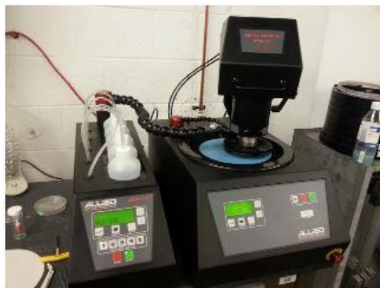
Fig 3.6 – Automatic polishing machine used for metallographic preparation: Allied MetPrep 3 Grinder/Polisher with Power Head (right) and AD-5 Fluid Dispenser (left)
