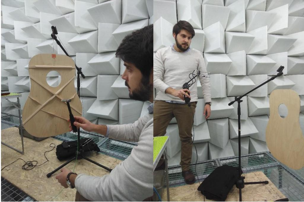
*Figure 3.3 b) – An example of the hammering and measuring during the tests.*
