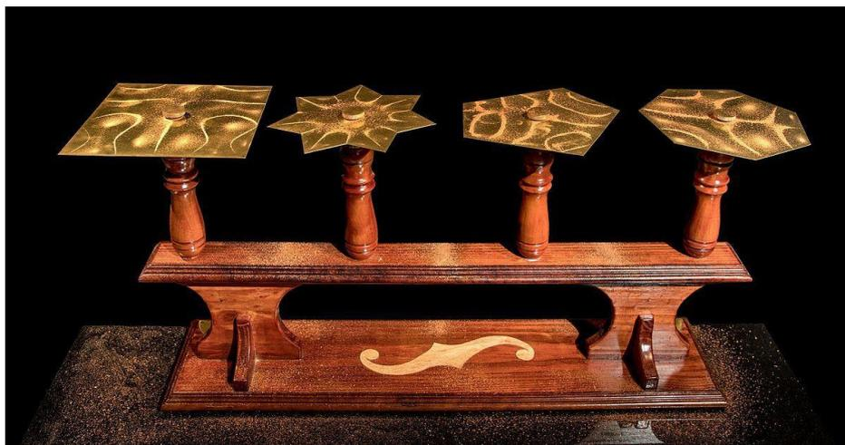
Figure 4.8 - Reproduction of the original Chladni layout.
