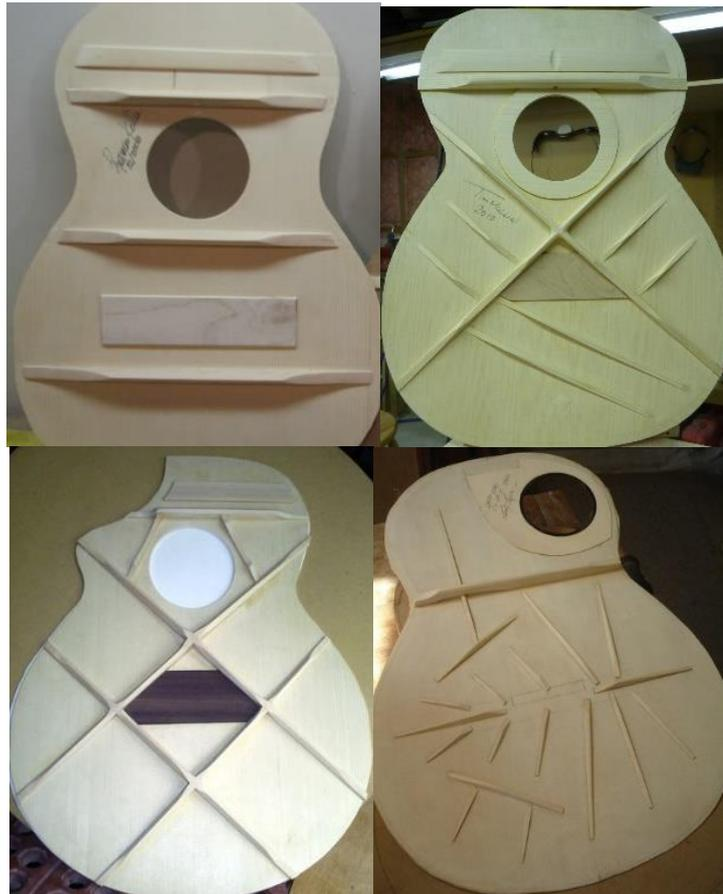
Figure 1.8 – From top-left to bottom-right: ladder, 'X', double 'X', and an asymmetrical pattern.
