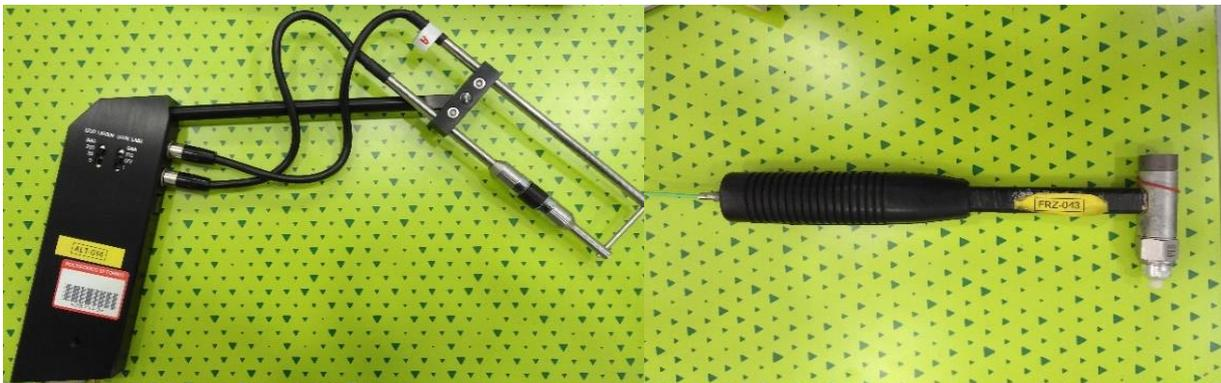
*Figure 3.2 a) – Intensimetric probe and instrumented hammer.*
