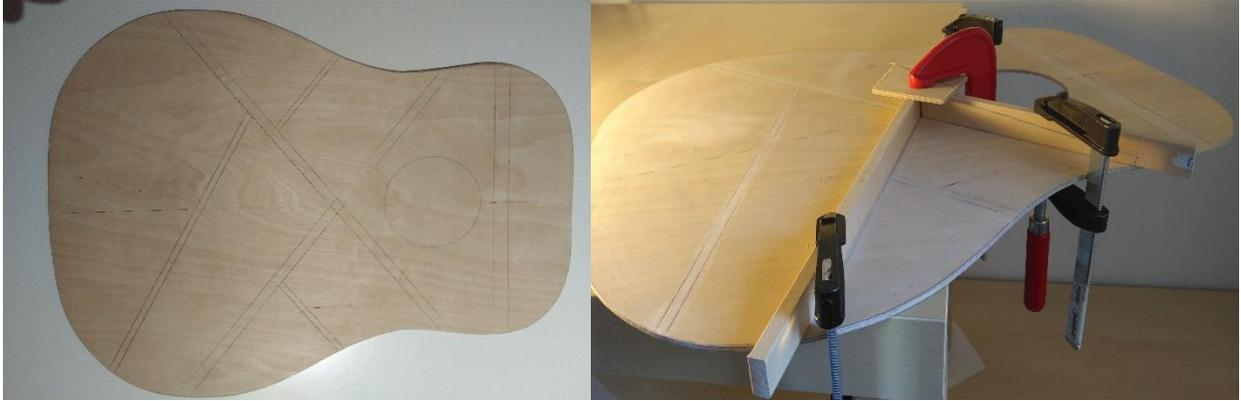
*Figure 3.7 – Bracing pattern reported on the soundboard; a phase of the gluing.*
