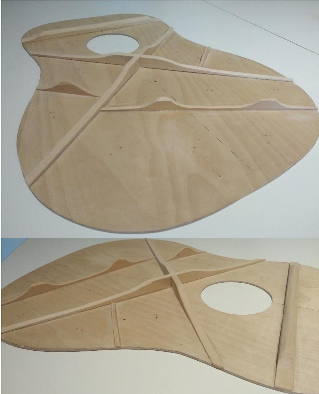
*Figure 3.16 – A detail of the scalloped bracing.*
