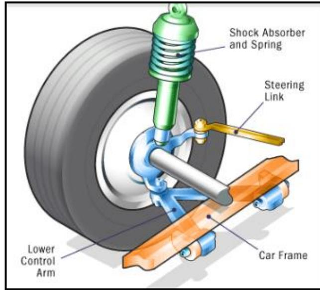
**Figure 5:** Basic Strut Design for a Suspension System [8]
