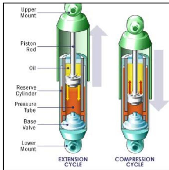
**Figure 4:** Twin-Tube Shock Absorber [8]
