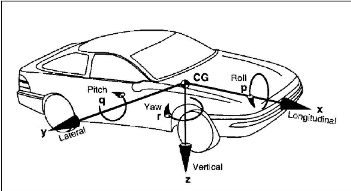
**Figure 2:** Vehicle Axis System [9]
