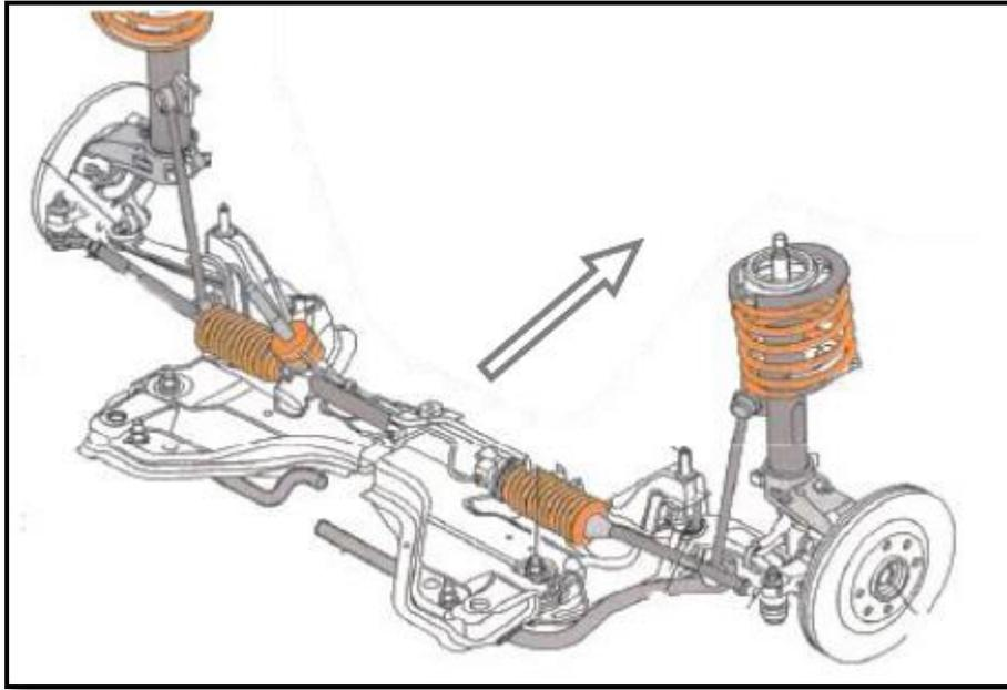
**Figure 6** : McPherson Front Suspension System
