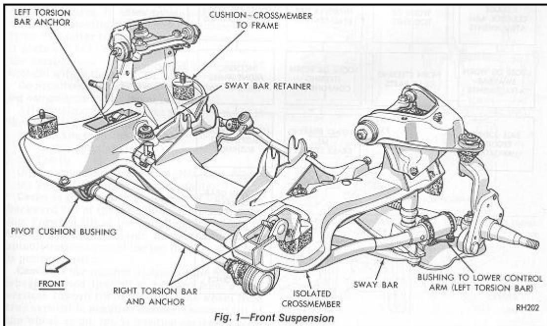
**Figure 13 :** Cradle (Cross Member) Model of a Car
