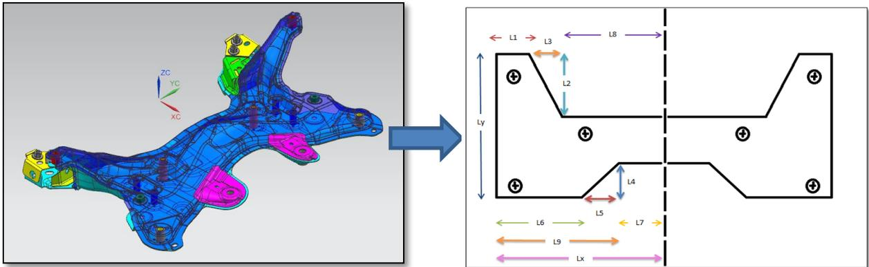
In order to make the calculations and the formation of the stiffness formulation easier, the actual cradle geometry is simplified as it is illustrated above. The model is composed of two symmetrical sheet metal geometries with a certain sheet metal thickness. Then the part will be completed with the addition of filler material on the inner side (which is neglected for the stiffness calculation of the cradle).
