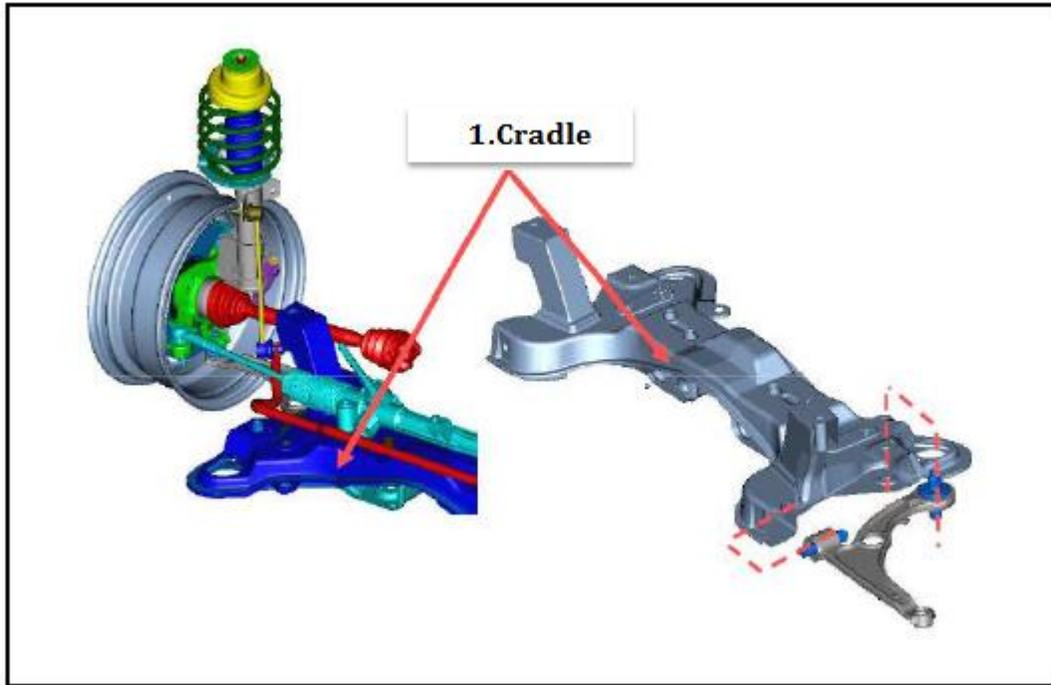
**Figure 7 :** Cradle (*Cross-member*) in the McPherson Suspension Model-I
