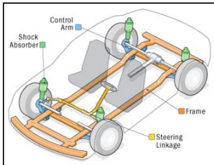
**Figure 1:** Chassis of a Car Body [8]
