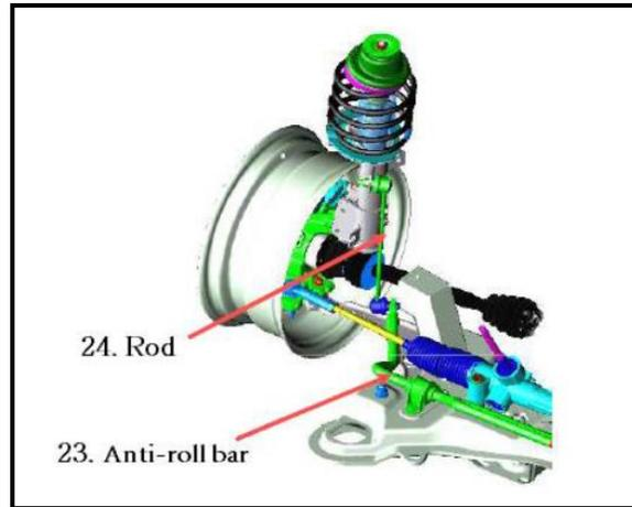
**Figure 11** : Front Wheel in the McPherson Suspension Model-V
