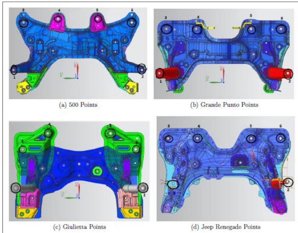
**Figure 25:** Six Attachment Points on the Cradle for Different Models
