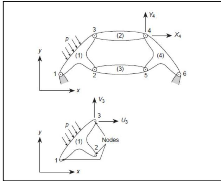
**Figure 26 :** Generic Discretization into Elements of a Structural Component
