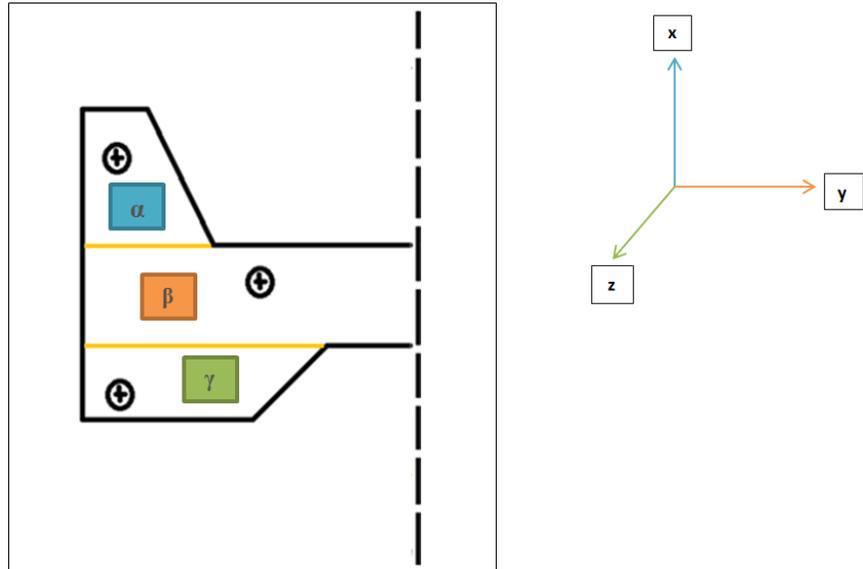
**Figure 32:** Half of the Symmetrical Simplified Cradle Model Divided into Three Areas for Second Formulation
