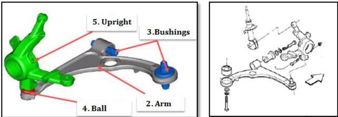
**Figure 8 :** Description of McPherson Suspension Model-II
