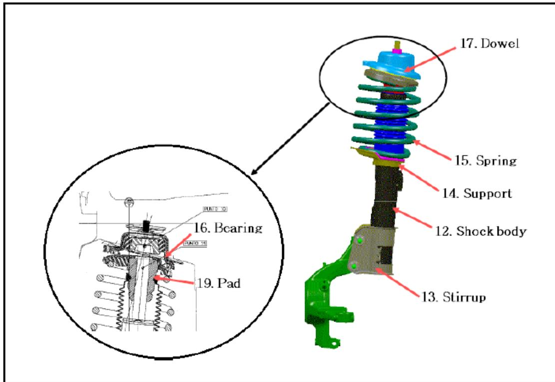
**Figure 10** : Shock Absorber in the McPherson Suspension Model-IV
