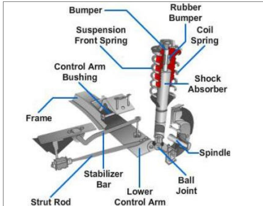
**Figure 3:** The basic components of a suspension system [11]
