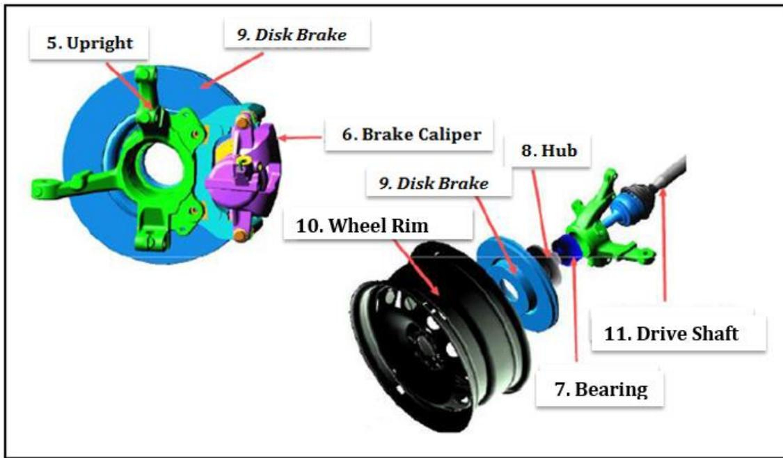
**Figure 9** : Description of McPherson Suspension Model-III
