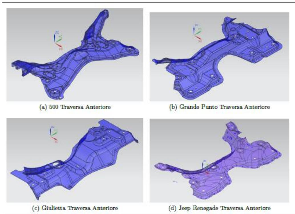
**Figure 24:** Front Cradle – Upper Shell Design
