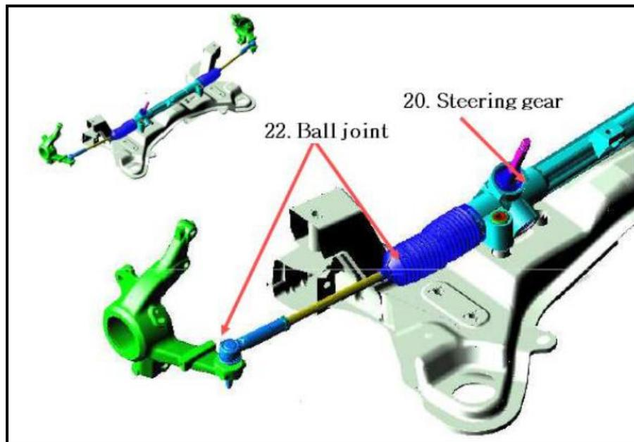
**Figure 12** : Steering Gear in the McPherson Suspension Model-VI
