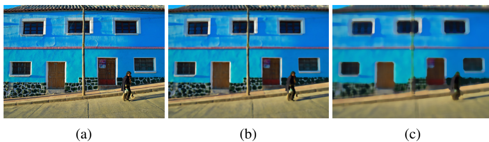
Fig. 2.7 Median filter with the different sizes of the Kernel matrix: (a) 3x3 Kernel, (b) 11x11 Kernel, (c) 25x25 Kernel.
