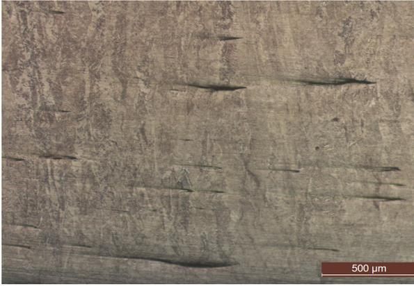
Figure 34 Unmelted zones at the bottom part of the sample "a"
