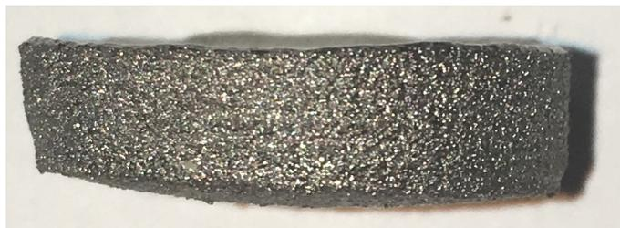
*Figure 22 Sample "a" after removing supports..*
