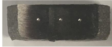
Figure 67 Three Macro indentation tests at 300 N on the real specimen .
