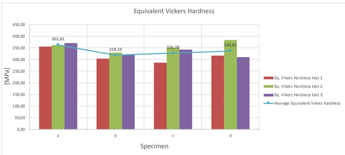
Figure 77 Scheme of the equivalent Vickers Hardness.
