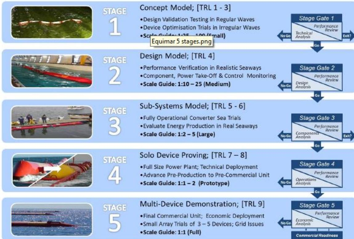
Figure 9: The 5 stages of development of a WEC proposed by Equimar
