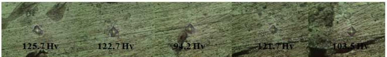
Figure 90: Hardness of diffusion zone in the joining seam of AFS composite
