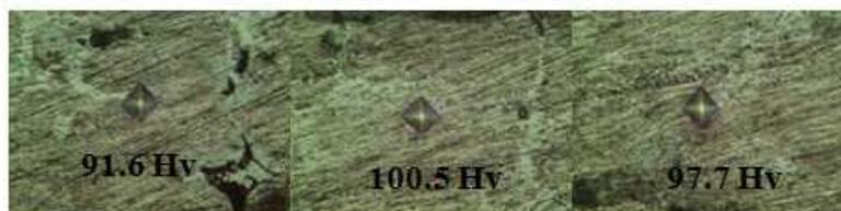
Figure 91: Micro Hardness of Al-Foam on the joining seam of AFS composite
