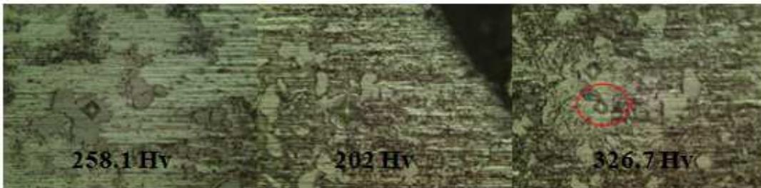
Figure 140: Phase 1 of brazed heat treated Al-Foam
