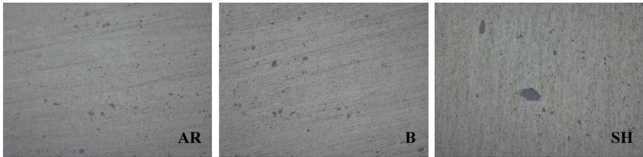
Figure 68: Microstructures as received (AR-left), brazed heat treated (B-middle), solution heat treated (SH-right) with 50x-1.25x magnification
