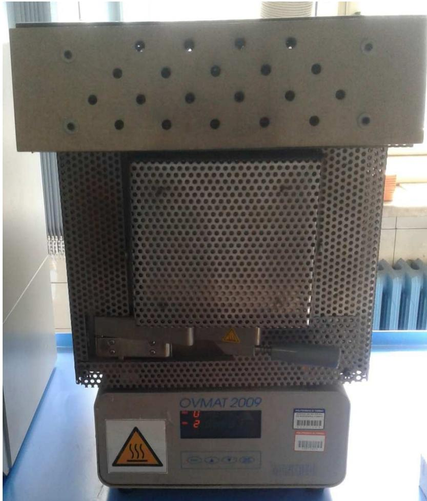
Figure 24: Solution heat treatment furnace for 1<sup>st</sup> batch of Al-7046 plates
