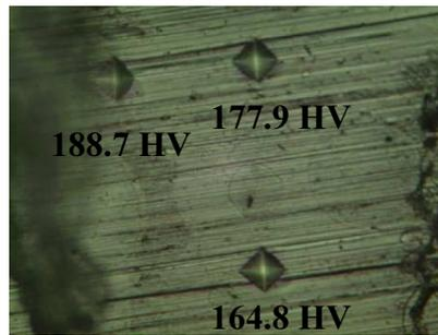
Figure 96: Hardness of diffusion zone in the joining seam of AFS composite
