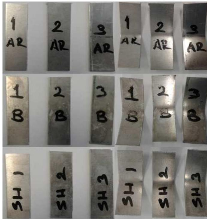
Figure 65: 3 point bending test for 2<sup>nd</sup> batch of Al-7046, left before, right after
