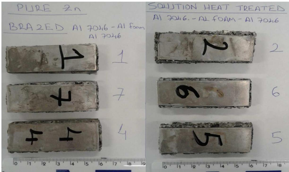
Figure 57: AFS composites with pure Zn before 3 point bending test
