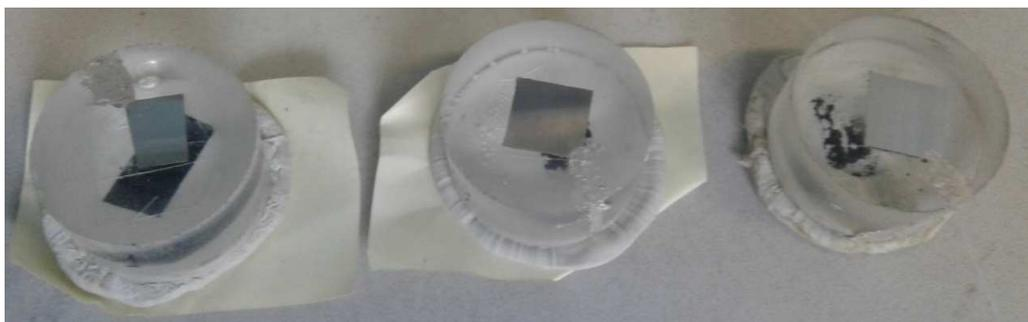
Figure 35: Epoxy kitt was applied on the bottom surface of glossed coated samples
