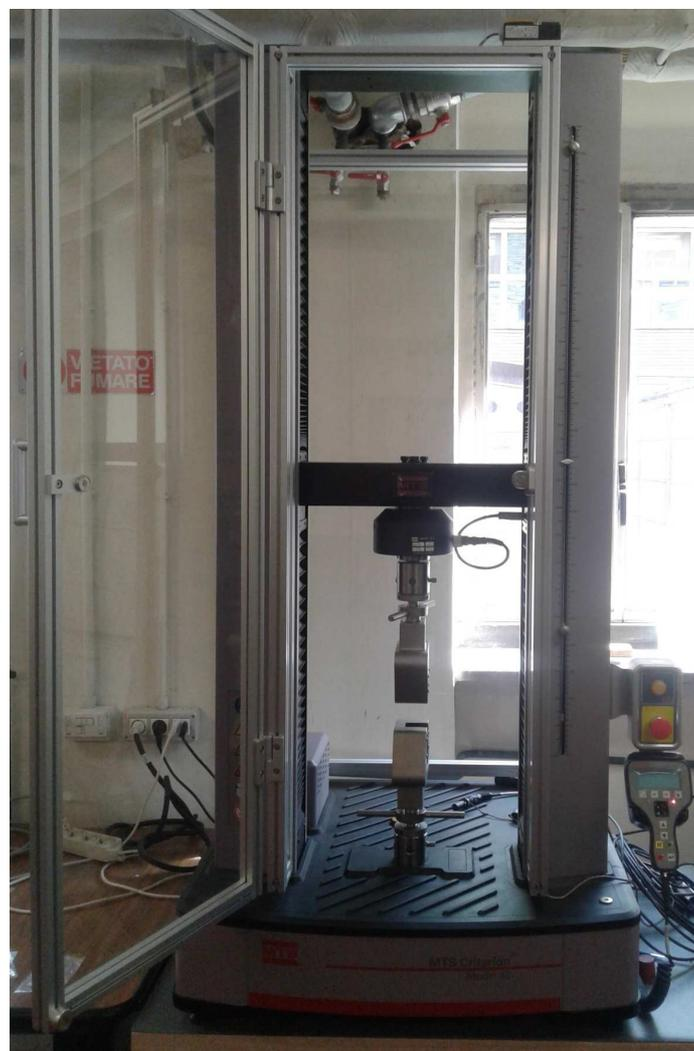
Figure 41: 3 point bending test machine
