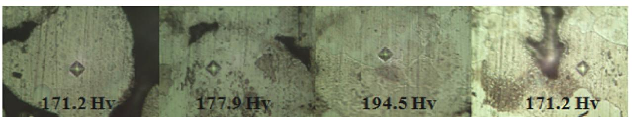
Figure 119: Micro Hardness of Al-Foam on the joining seam of AFS composite
