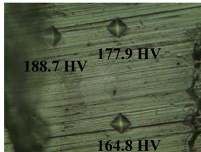
Figure 96: Hardness of diffusion zone in the joining seam of AFS composite
