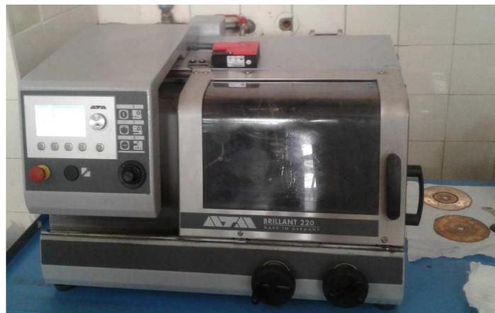
Figure 148: Ata Brillant 220 cutting machine
