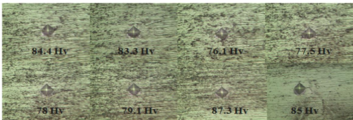
Figure 115: Micro Hardness of Al-plate edge of the joining seam of AFS composite
