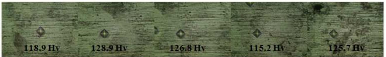
Figure 139: Matrix form of brazed heat treated Al-Foam
