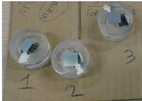
Figure 28: Silver liquid was applied on the gloss coated samples
