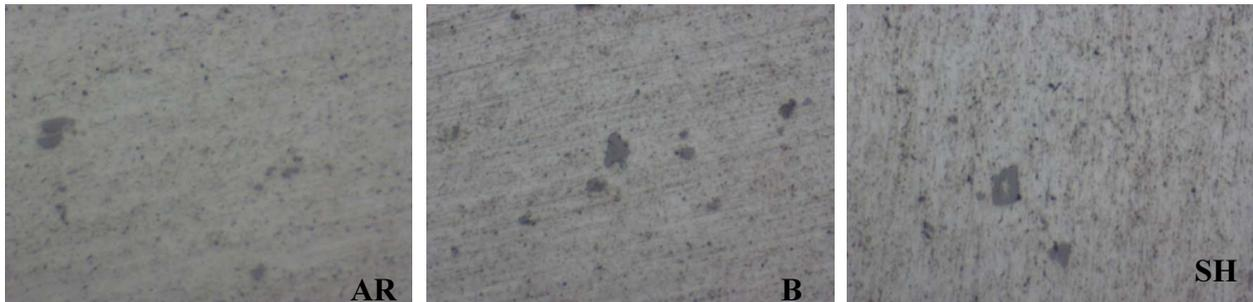
Figure 66: Microstructures as received (AR-left), brazed heat treated (B-middle), solution heat treated (SH-right) with 100x-1.88x magnification
