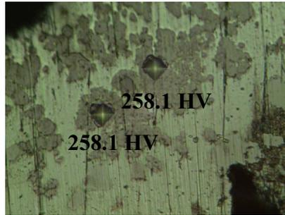
Figure 144: Phase 1 of solution heat treated Al-Foam
