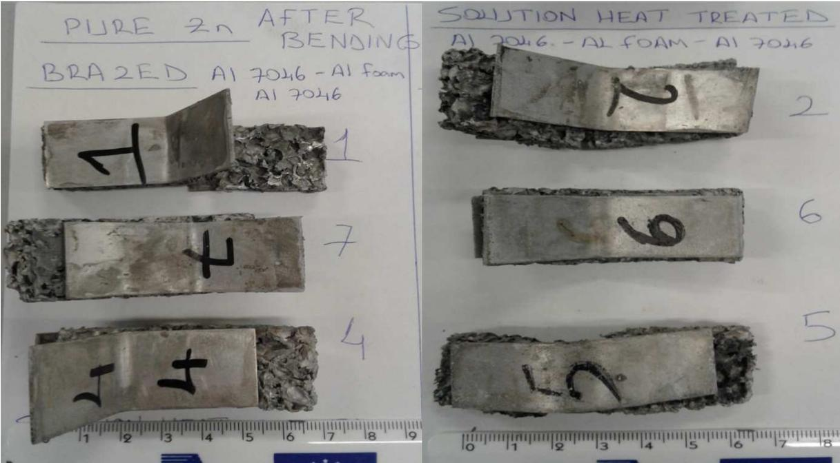
Figure 61: AFS composites with pure Zn after 3 point bending test
