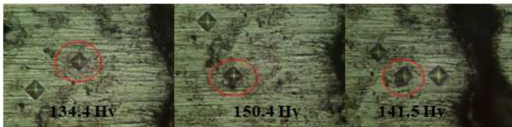
Figure 141: Mixture form of brazed heat treated Al-Foam
