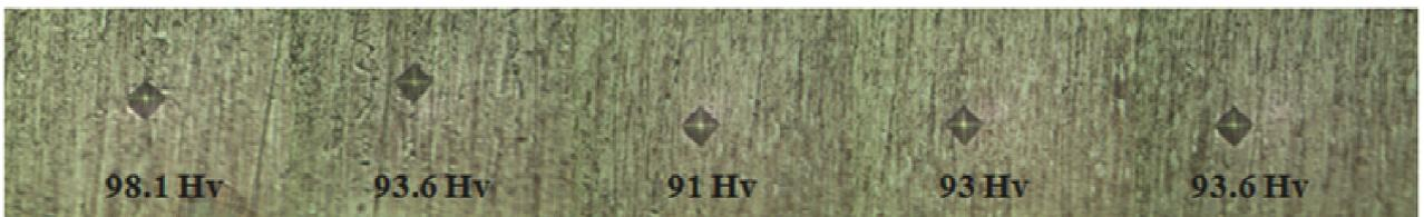
Figure 118: Micro Hardness of Al-plate edge of the joining seam of AFS composite
