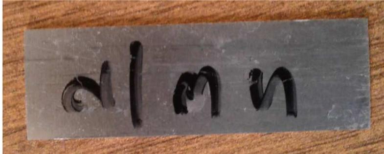
Figure 39: Brazed heat treated Al-7046 before 3 point bending
