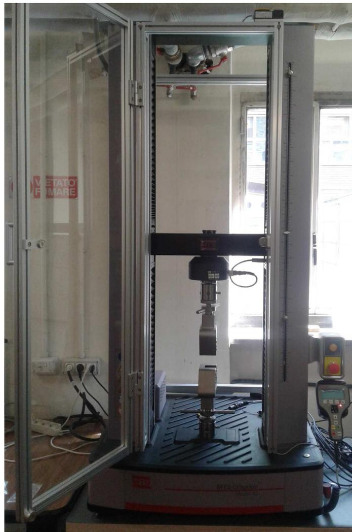
Figure 41: 3 point bending test machine
