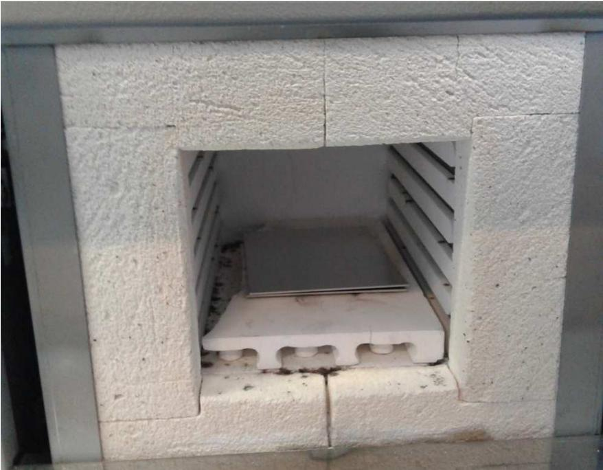
Figure 21: Locating the Al as received plates in the furnace
