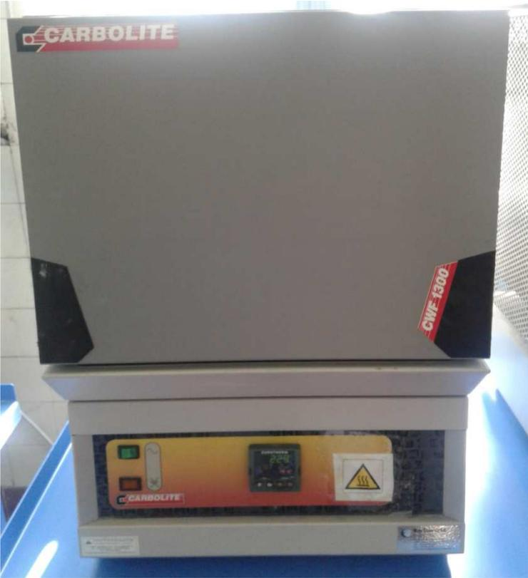
Figure 20: Brazing heat treatment furnace for 1<sup>st</sup> batch of Al-7046 plates
