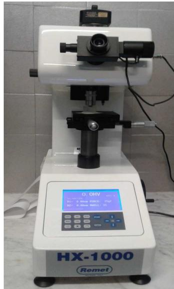
Figure 36: Vickers micro-hardness instrument
