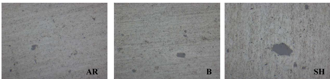
Figure 67: Microstructures as received (AR-left), brazed heat treated (B-middle), solution heat treated (SH-right) with 100x-1.25x magnification
