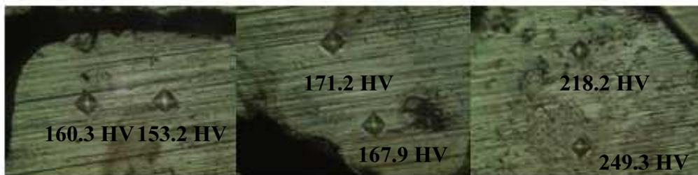
Figure 97: Micro Hardness of Al-Foam on the joining seam of AFS composite
