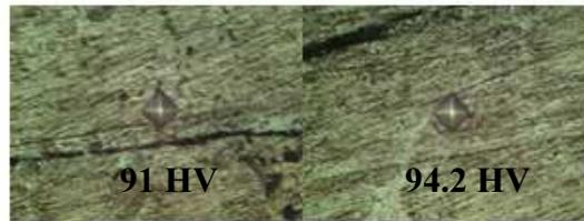
Figure 92: Micro Hardness of joint seam of AFS composite
