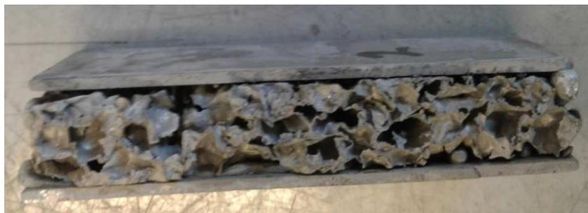
Figure 54: Result of the brazing parameters, AFS composite brazed with Zn2%Al
