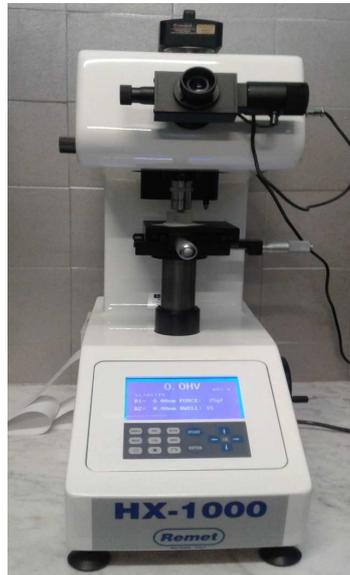
Figure 36: Vickers micro-hardness instrument
