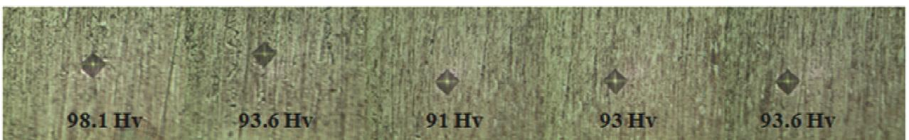
Figure 118: Micro Hardness of Al-plate edge of the joining seam of AFS composite
