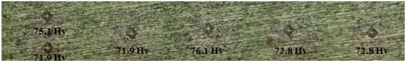
Figure 95: Micro Hardness of Al-plate edge of the joining seam of AFS
