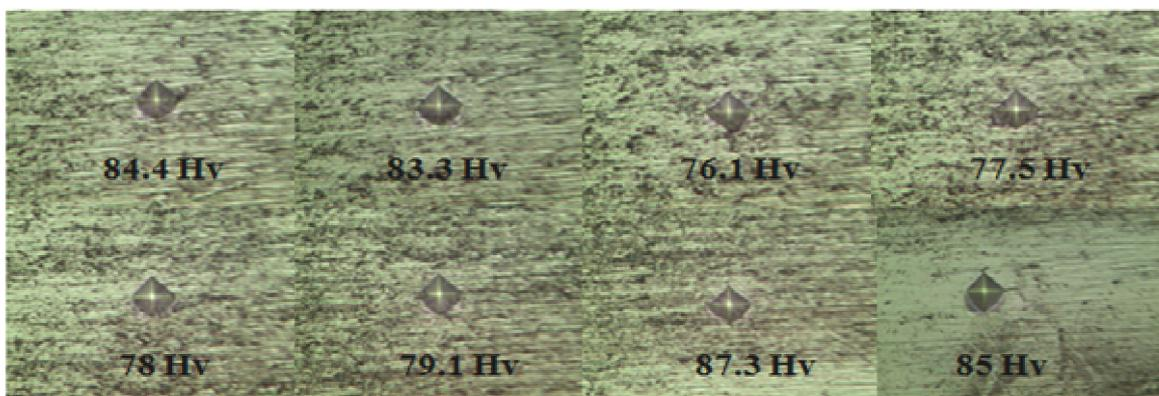
Figure 115: Micro Hardness of Al-plate edge of the joining seam of AFS composite
