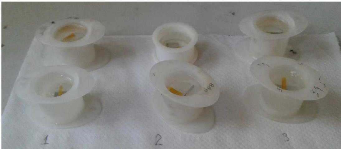
Figure 26: Gloss coated samples in the mixture of epoxy resin and hardener
