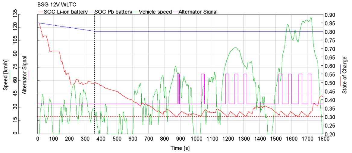
Figure 29: SOC, vehicle speed and alternator mode signal for BSG model (WLTC).
