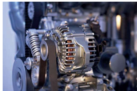
Figure 20. Installation of Valeo BSG 12V
