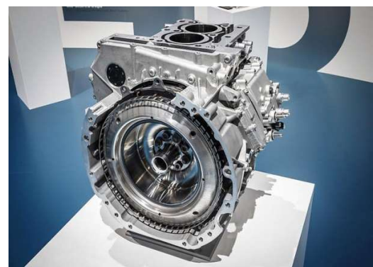
Figure 27. P2 coaxial application by Mercedes-Benz
