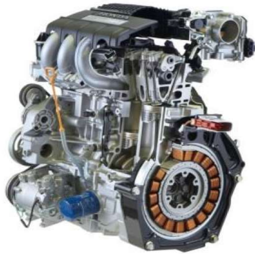
Figure 22. Integrated Motor Assist (IMA) by Honda
