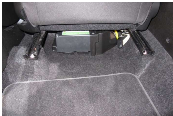
Figure 53. Installation of Lithium-Ion Battery
