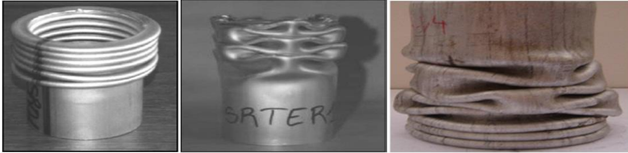
Figure 22 – Left to right: concertina mode, diamond mode and mix mode deformation
