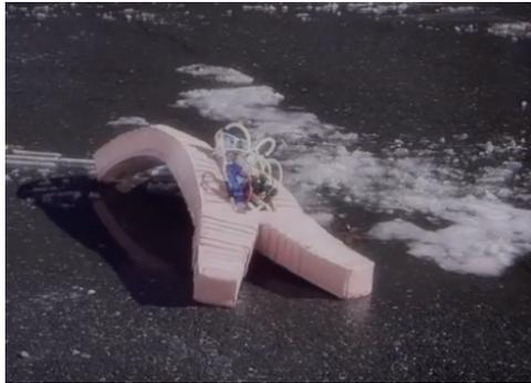
Figura 4.5: Soft robot in gomma siliconica
