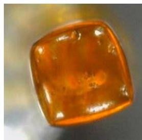
(c) Top-view of fabricated structure consisting 30  $\mu\text{m}$  thick layers followed by a base layer and squares of sizes 300x300, 250x250 and 200x200 pixels.
