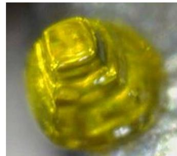
(b) Top view of fabricated structure consisting 10  $\mu\text{m}$  thick layers followed by a base layer and squares of sizes 200x200, 150x150 and 100x100 pixels.
