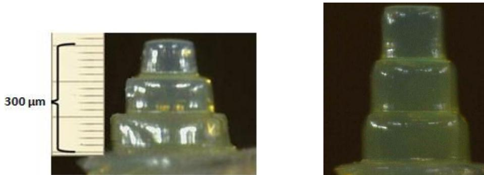
(a) Fabricated structure consisting 10  $\mu\text{m}$  thick layers followed by a base layer and squares of sizes 200x200, 150x150 and 100x100 pixels.
