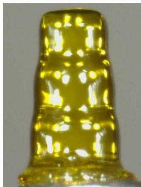
(c) Side-view of fabricated structure consisting 30  $\mu\text{m}$  thick layers followed by a base layer and squares of sizes 300x300, 250x250 and 200x200 pixels.
