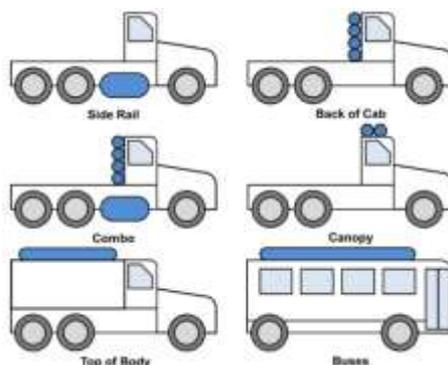
Figure 2.20: Design of storage space for medium and heavy-duty vehicles [10]
