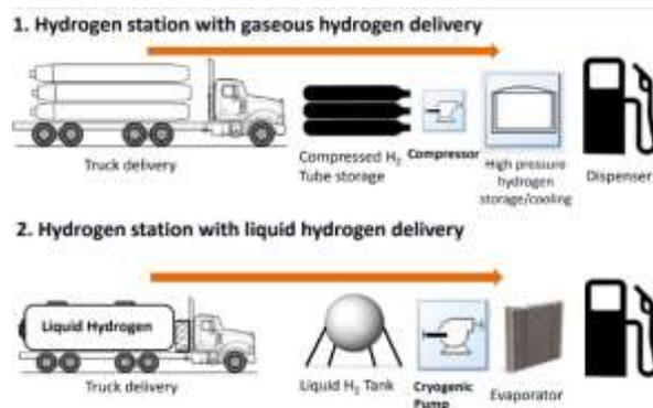
Figure 4.4: Hydrogen delivery: Station Configuration [38]
