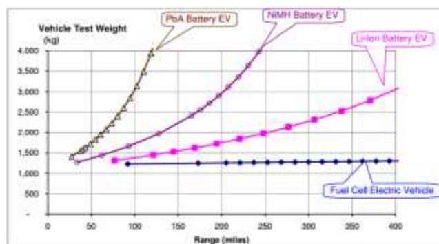
Figure 2.9: Weight increase with respect to range for light-duty vehicle application, the power trains are designed to provide a 0-97km/h acceleration in 10s
