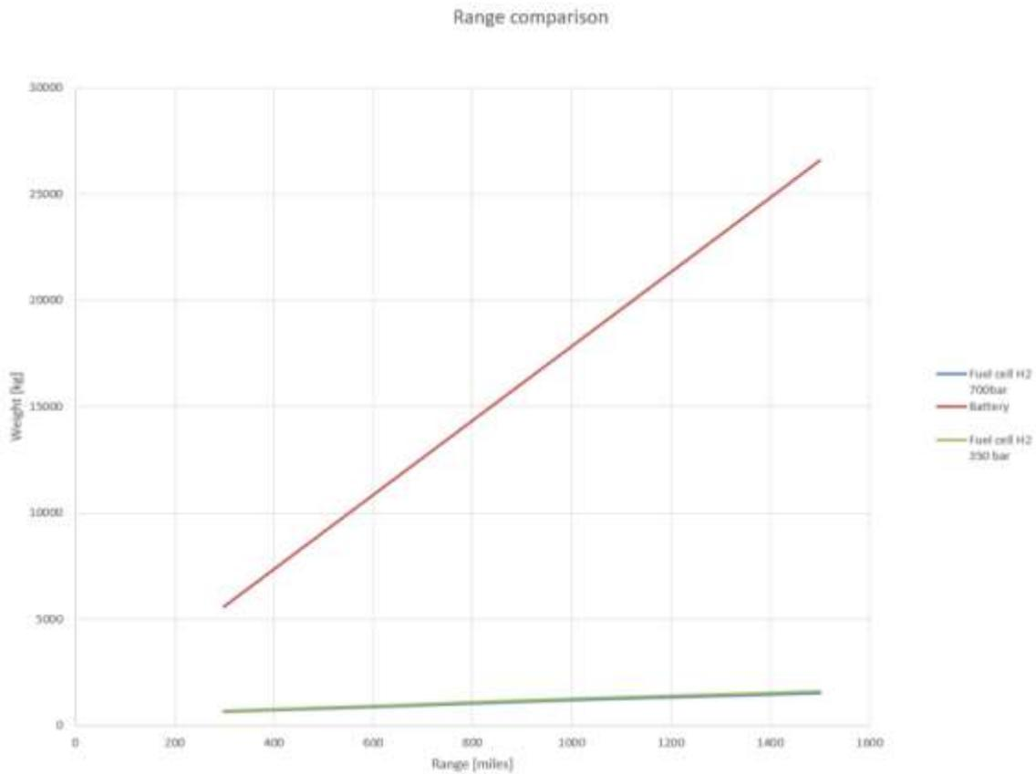
Figure 2.23: Weight of battery and fuel cell system compared increasing range
