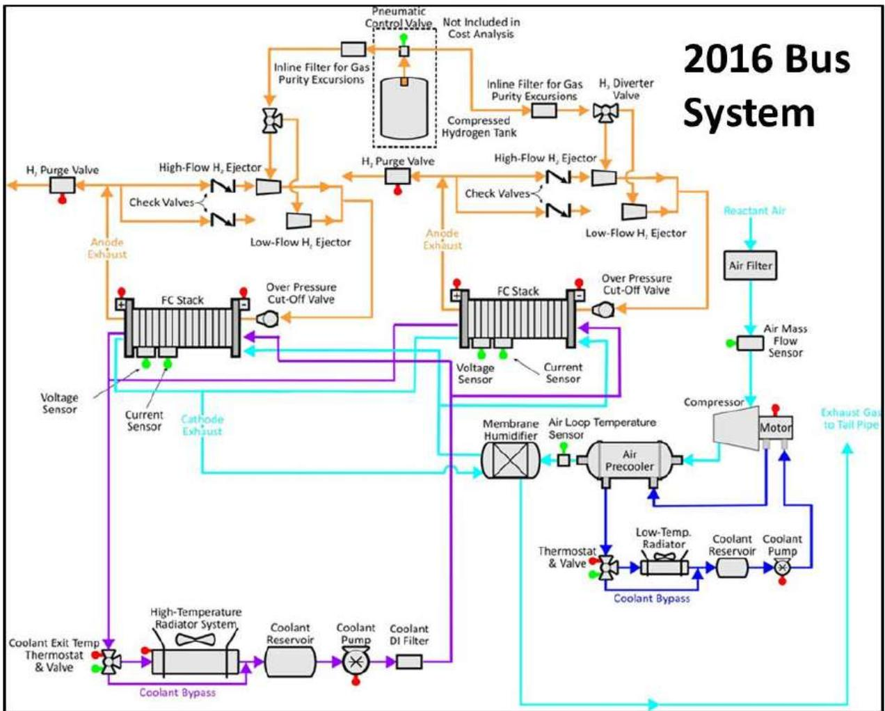
Figure 4.2 Flow schematic for the bus fuel cell system
