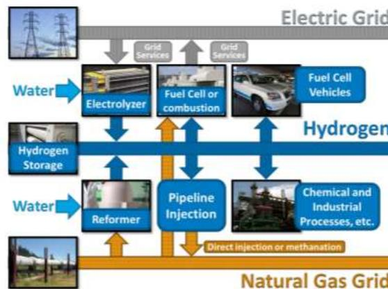
Figure 2.16 Hydrogen technologies configurations
