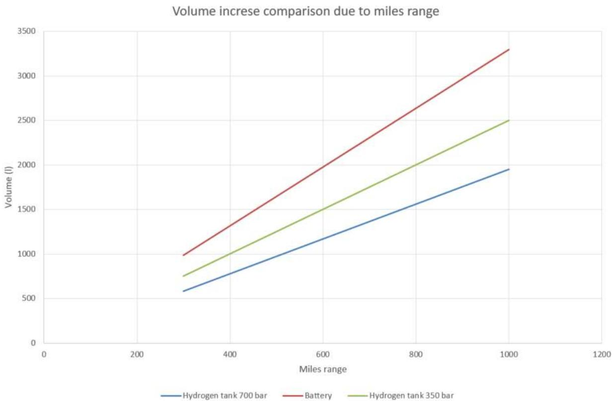
Figure 2.24: Volume of battery and hydrogen tank compared increasing range
