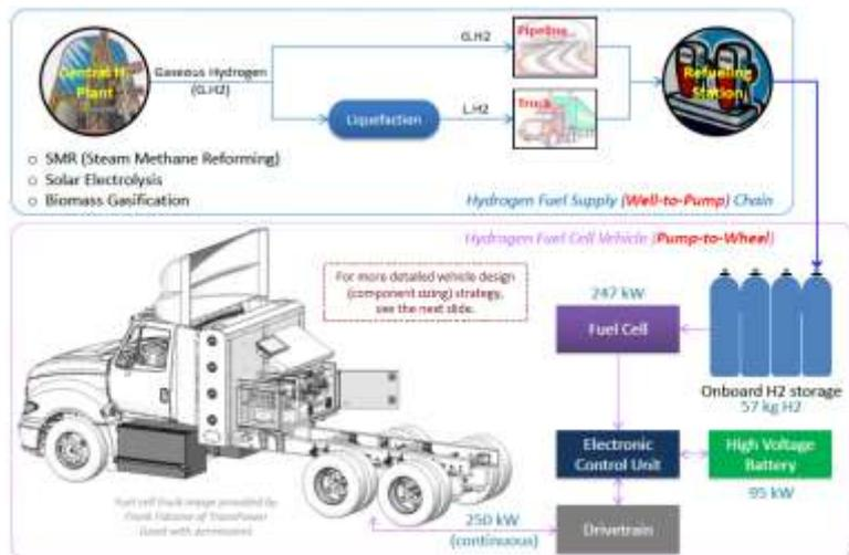
Figure 4.1: Medium and heavy-duty hydrogen fuel cell truck system configuration [28]
