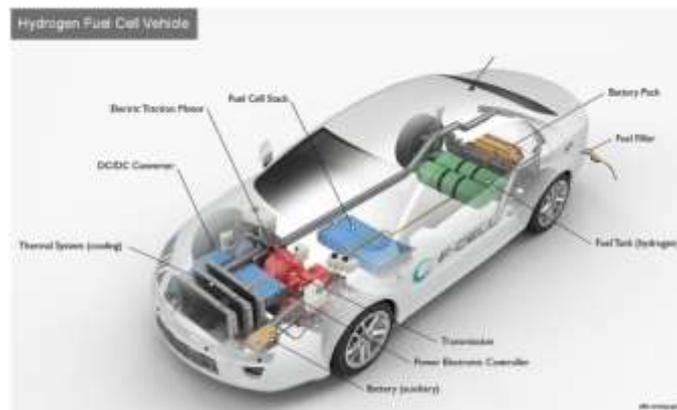
Figure 2.8: Fuel cell vehicle components detail [33]
