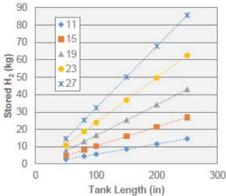
Figure 2.14 Mass of stored Hydrogen with respect to tank dimension for 700bar case. Each color and shape correspond to a constant diameter (in) [10]
