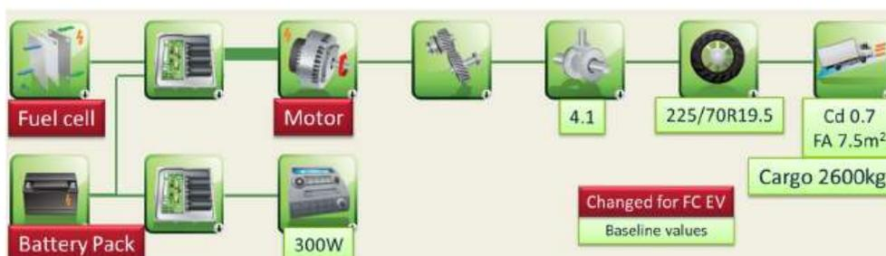
Figure 2.11 Schematic diagram for a medium fuel cell electric truck [9]
