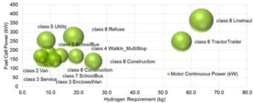
Figure 2.21: Fuel cell and hydrogen tank sizing for FCETs for guaranteeing the same performance as the baseline trucks [10]
