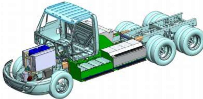
Figure 2.19: CAD modelling of a heavy-duty truck for emphasizing the amount of space available for FCET components
