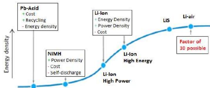
Figure 2.2 Gravimetric Energy Density of different battery chemistry [17]
