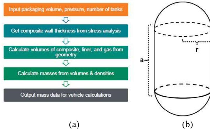
Figure 2.13 On-board truck hydrogen storage modelling flow chart (a) and capsule geometry typically used for Composite Overwrapped Pressure Vessels (COPV) (b) [10].
