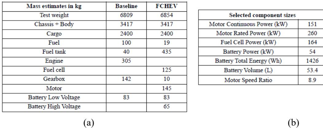
Figure 2.12 Mass difference between Baseline vehicle and FCET version (a) and result of the component dimension (b) [9]
