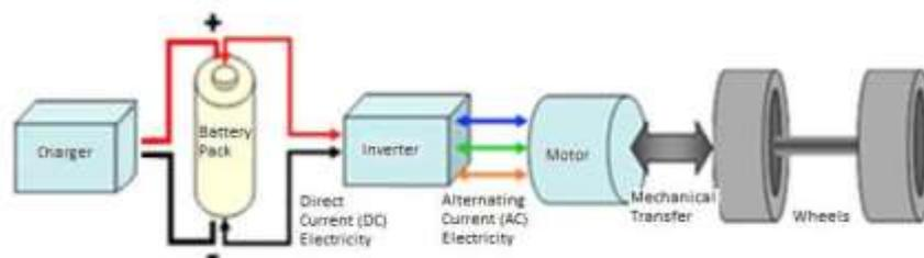
Figure 2.1 Simplistic overview of BEV components [17]
