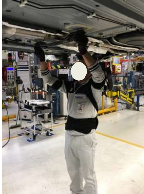
Figure 46 Workstation #3 (Assembly): Tunnel reinforcement bracket (Team Leader) [December 2017, FCA copyright]
