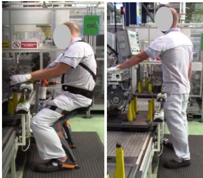
Figure 17 Chamfering tool assembly workstation with and without CC [August 2017, Bielsko Biala plant]
