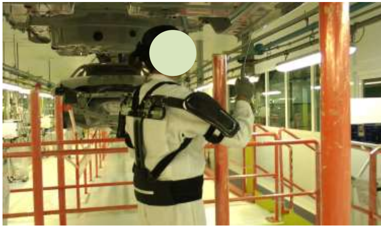
Figure 53 Workstation underbody sealing (OP004) - AGAP trial
