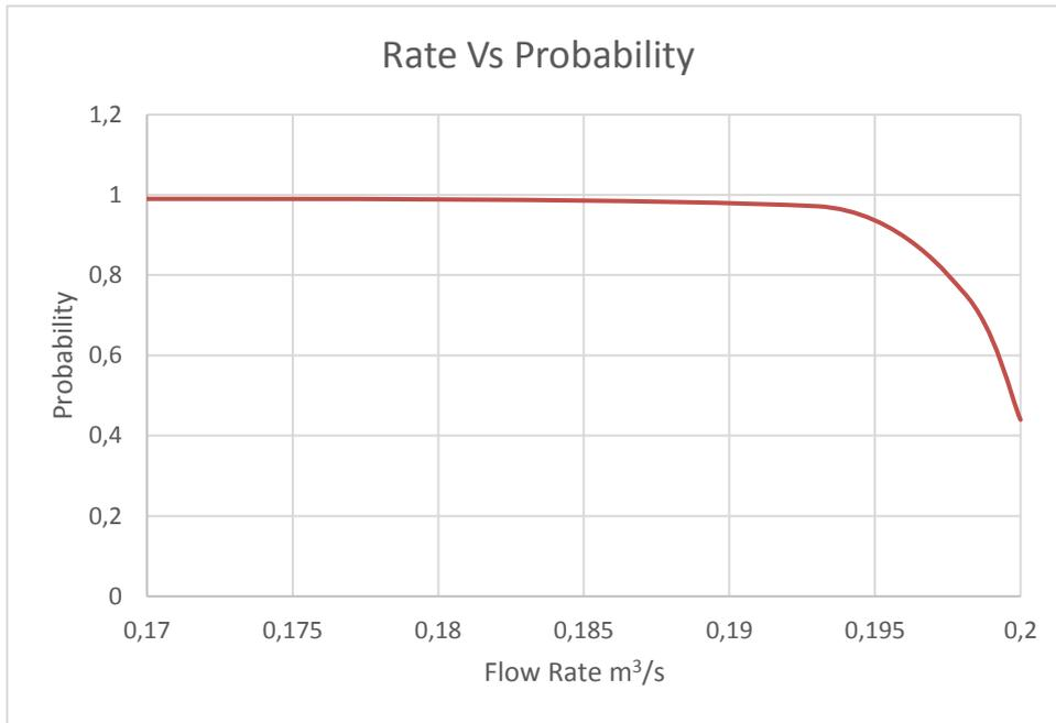
Figure 3.10: The probability of achieving a range of flow rates after failure for pump station 4
