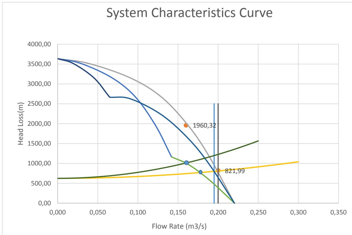
Figure 3.15: Pump Station 1 with 3 Pumps failed
