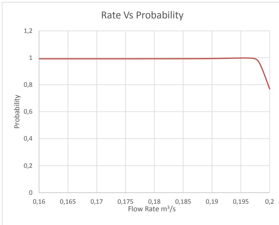
Figure 4.1: The probability of achieving a range of flow rates after failure for pump station 1 with additional pumps in series
