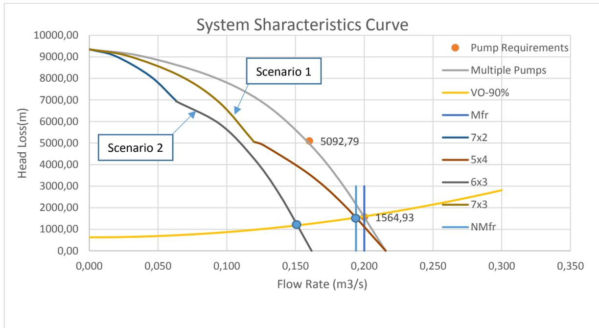
Figure 3.5: Pump Station 2 with 2 Pumps failed
