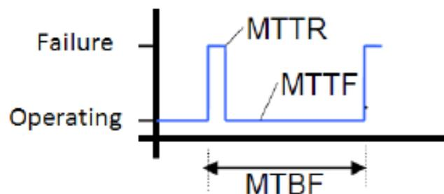
Figure 1.1: Failure vs time relation
