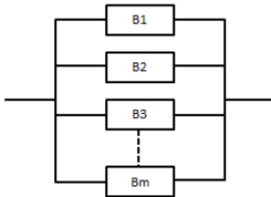
Figure 1.4: Reliability Block Diagram in Parallel
