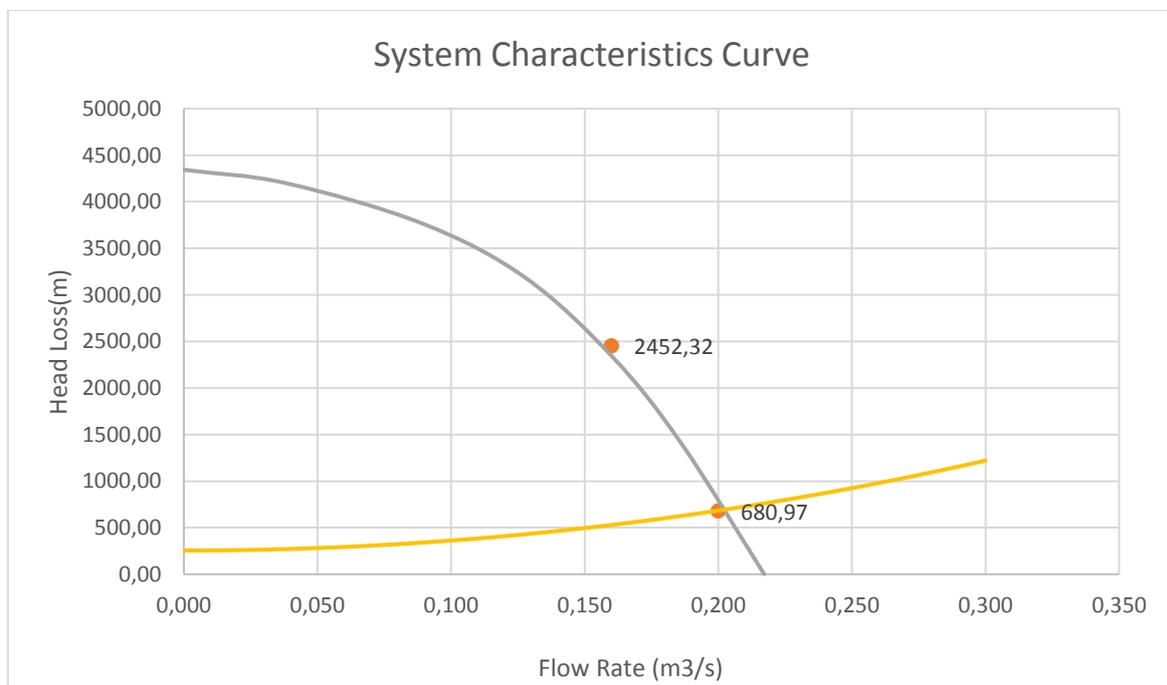
Figure 1.8. Sample pump system curves
