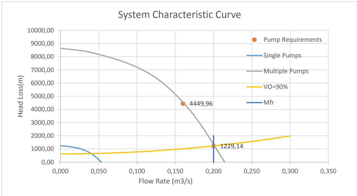
Figure 2.7: Characteristic Curve for Pump Station 3 at 90% Opening
