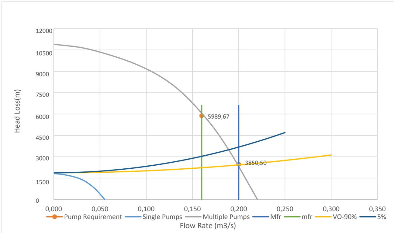
Figure 2.16: Characteristic Curve for Pump Station 1 (Scenario 3) at 90% Opening
