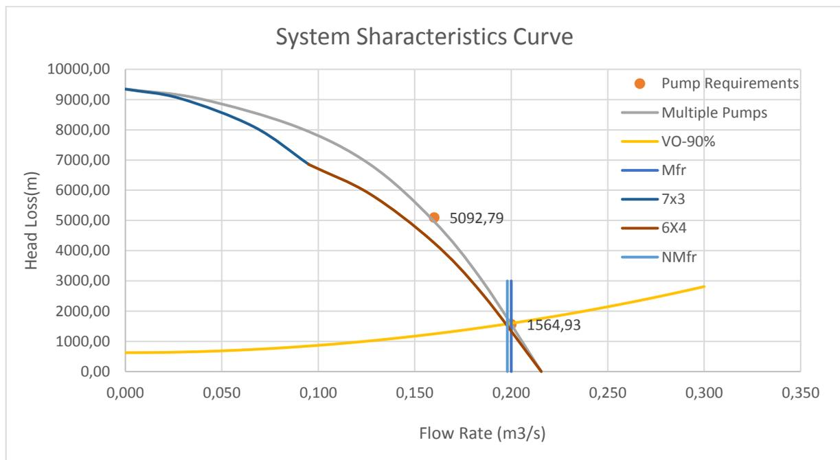
Figure 3.4: Pump Station 2 with 1 Pumps failed
