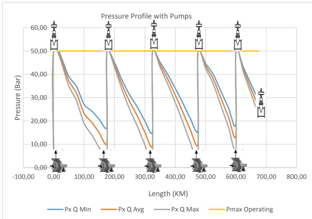
Figure 2.11: Pressure Profile Showing Pumping Stations
