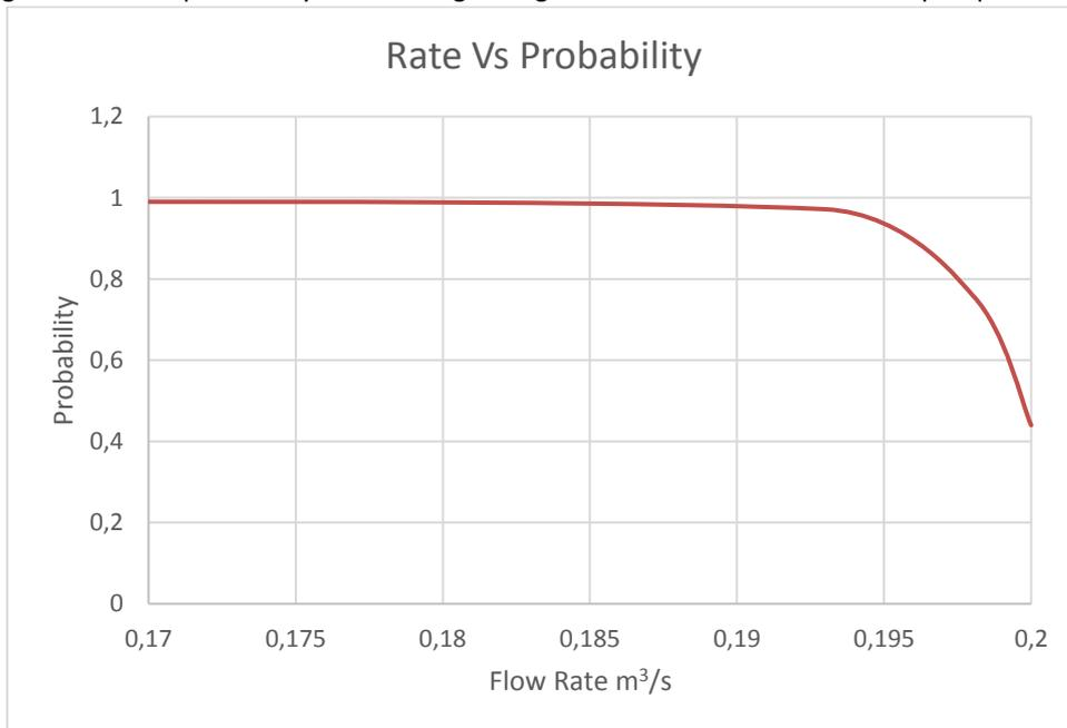
Figure 3.11: The probability of achieving a range of flow rates after failure for pump station 5
