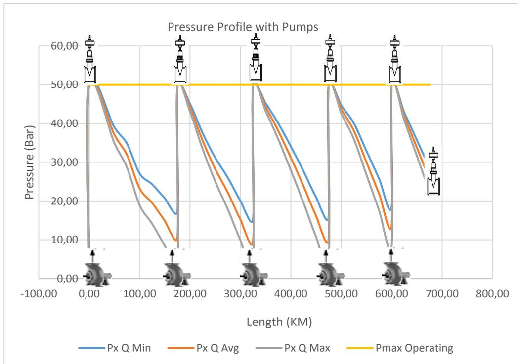
Figure 2.4: Pressure Profile Showing Pumping Stations
