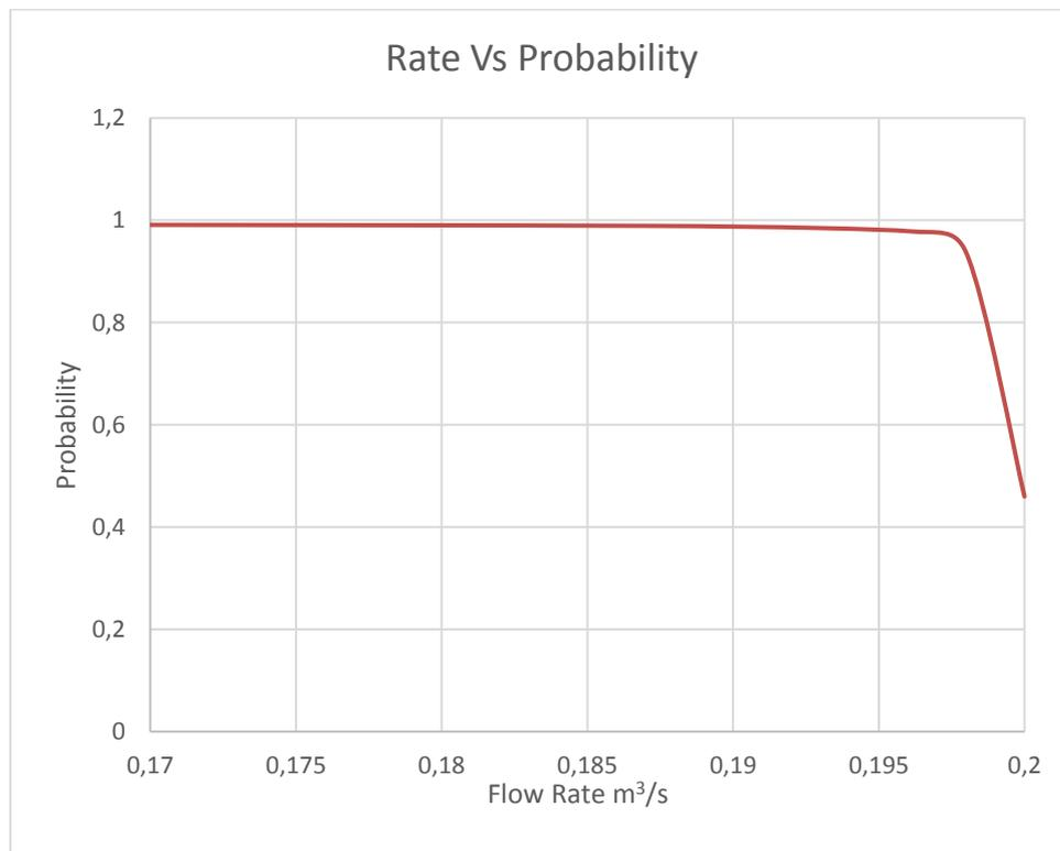
Figure 3.7: The probability of achieving a range of flow rates after failure for pump station 1
