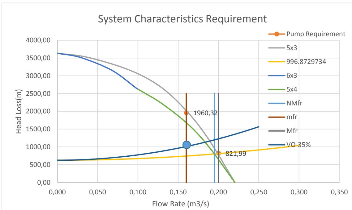
Figure 3.1: Pump Station 1 with 1 Pump failed
