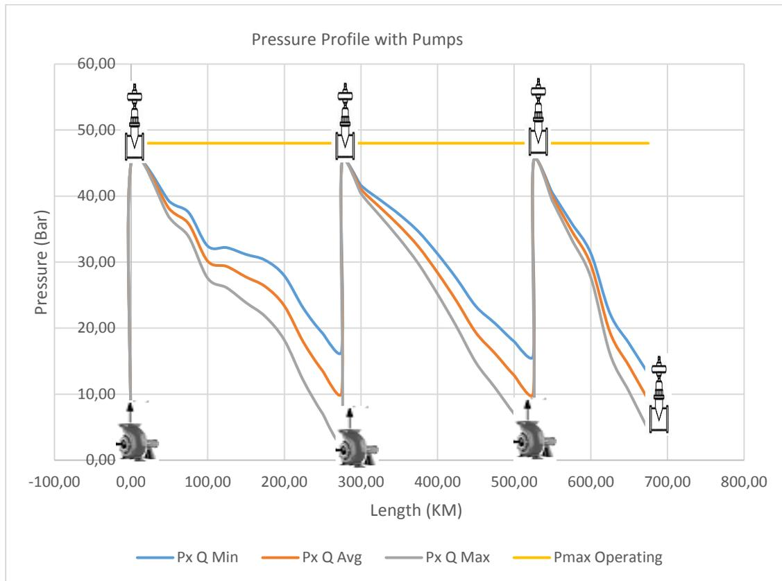
Figure 2.15: Pressure Profile Showing Pumping Stations
