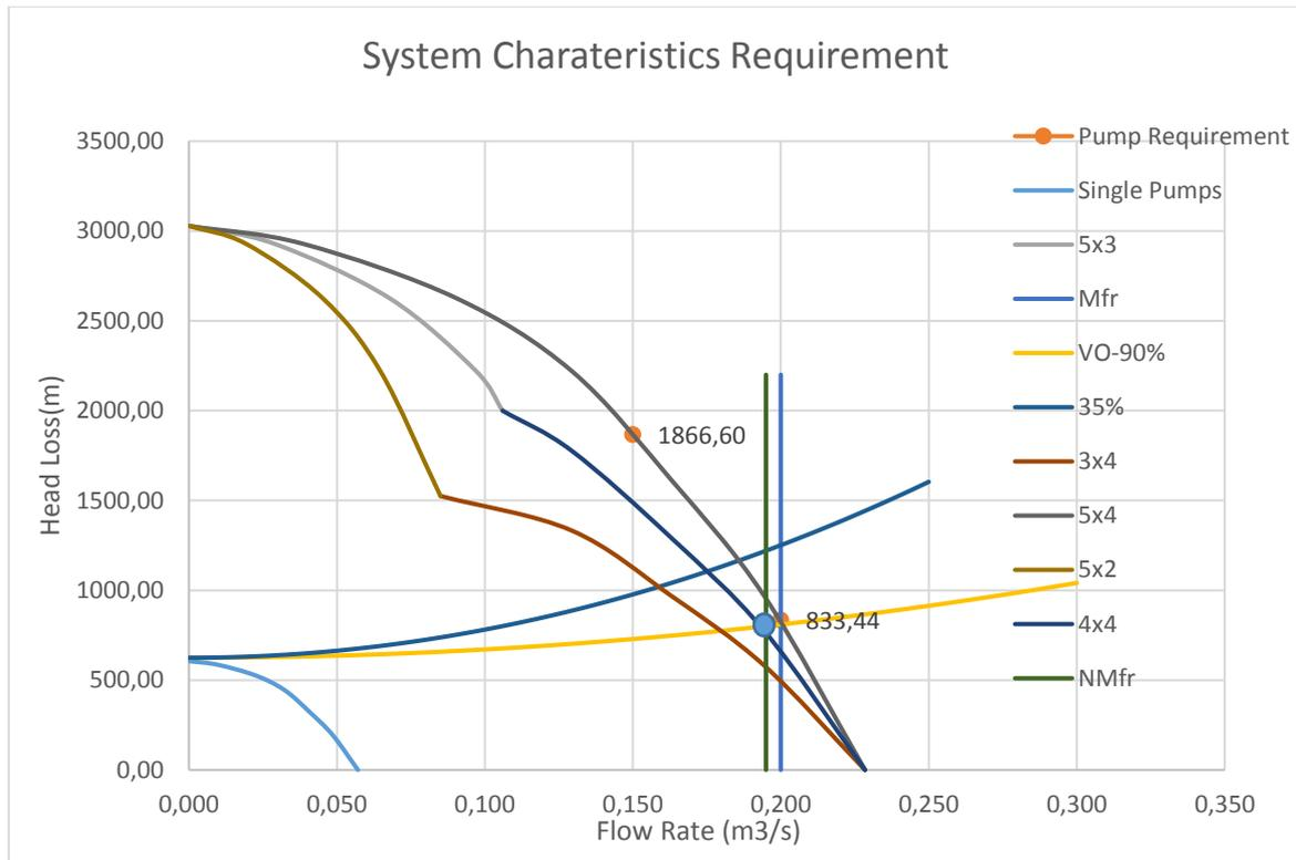
Figure 3.13: Pump Station 1 with 1 Pump failed
