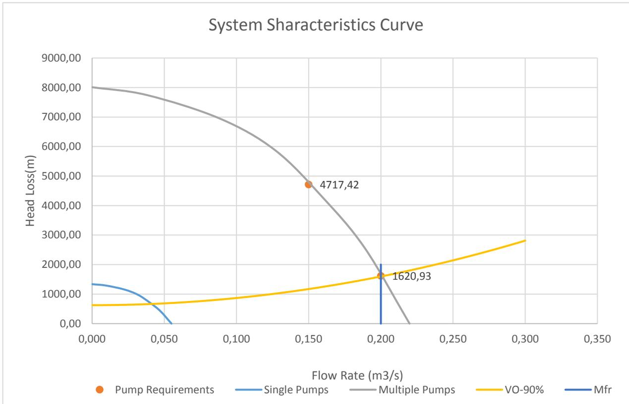
Figure 2.13: Characteristic Curve for Pump Station 2 (Scenario 2) at 90% Opening
