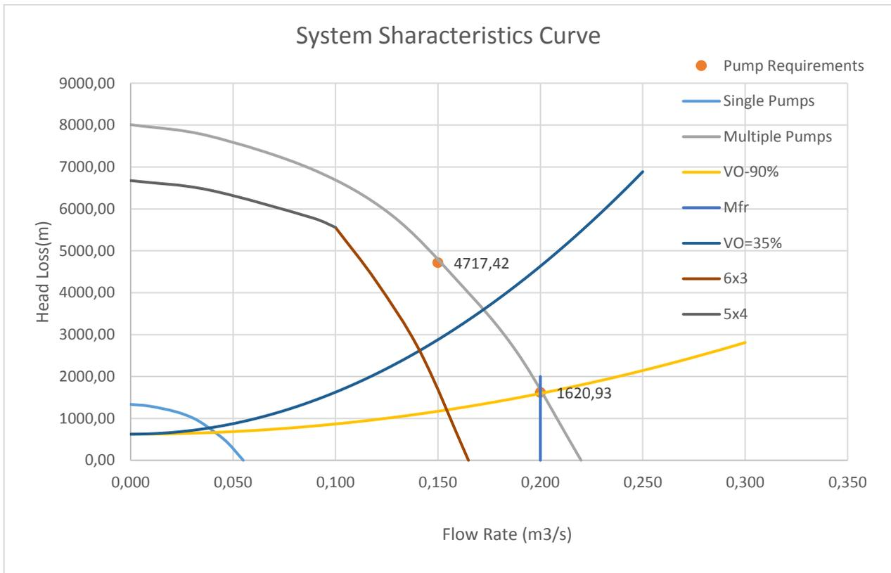
Figure 3.16: Pump Station 2 with 1 Pumps failed
