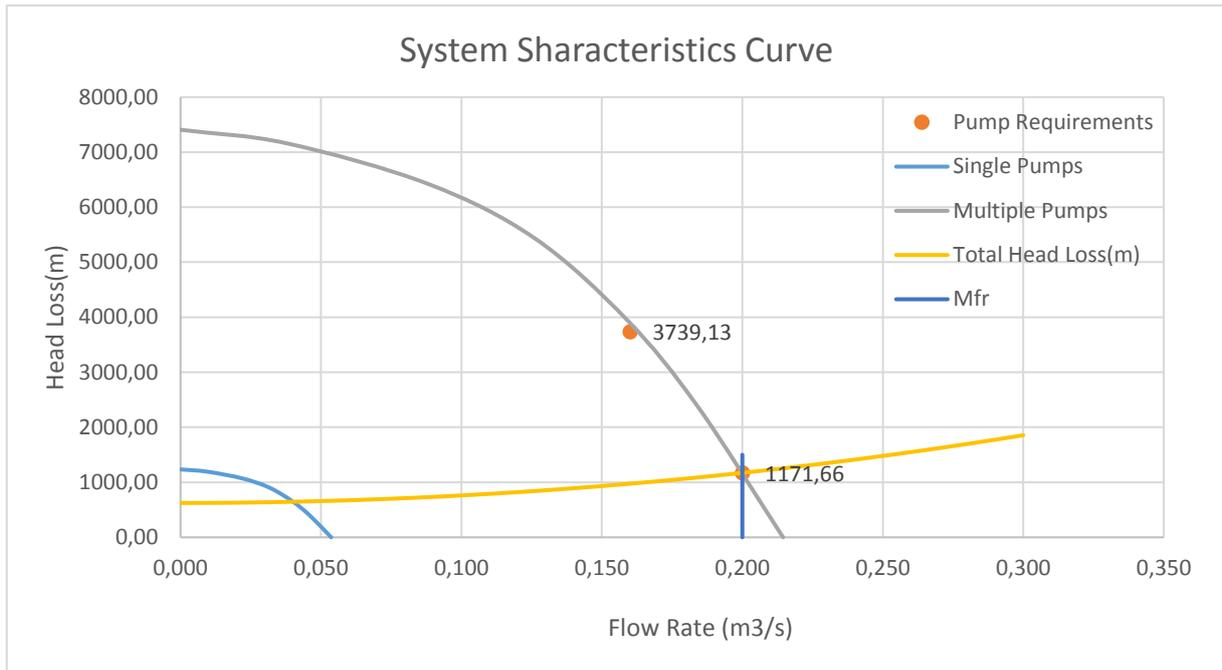
Figure 2.9: Characteristic Curve for Pump Station 5 at 90% Opening
