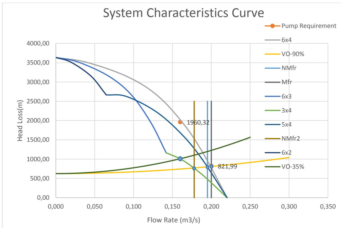
Figure 3.3: Pump Station 1 with 3 Pumps failed
