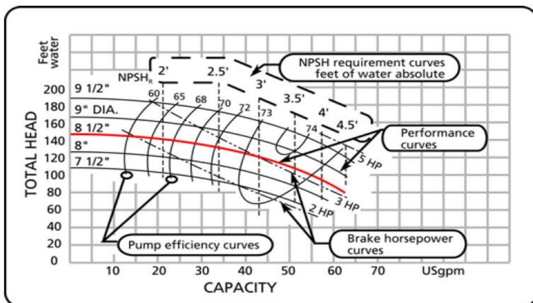
Figure 1.7. A Pump performance curve
