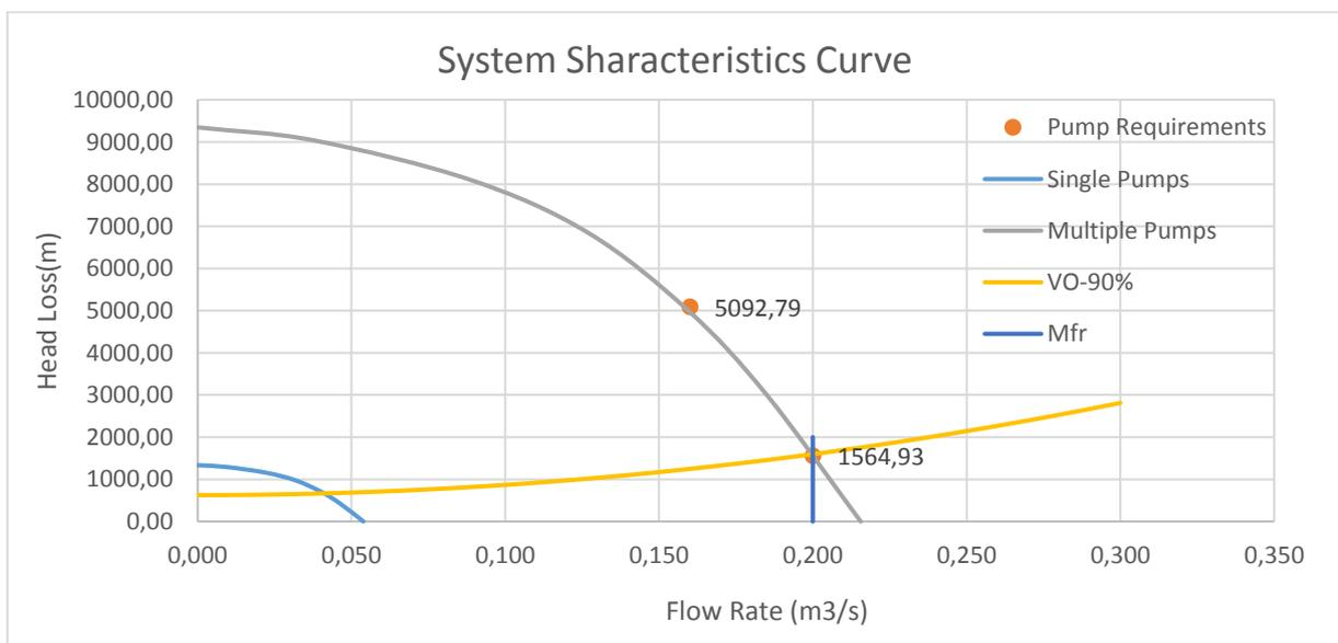
Figure 2.6: Characteristic Curve for Pump Station 2 at 90% Opening
