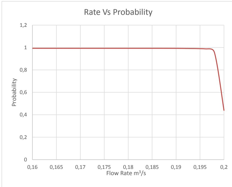
Figure 3.19: The probability of achieving a range of flow rates after failure for pump station 1
