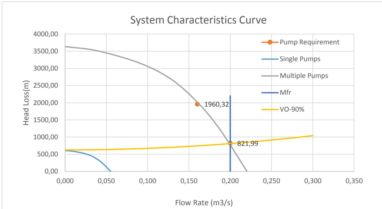
Figure 2.5: Characteristic Curve for Pump Station 1 at 90% Opening
