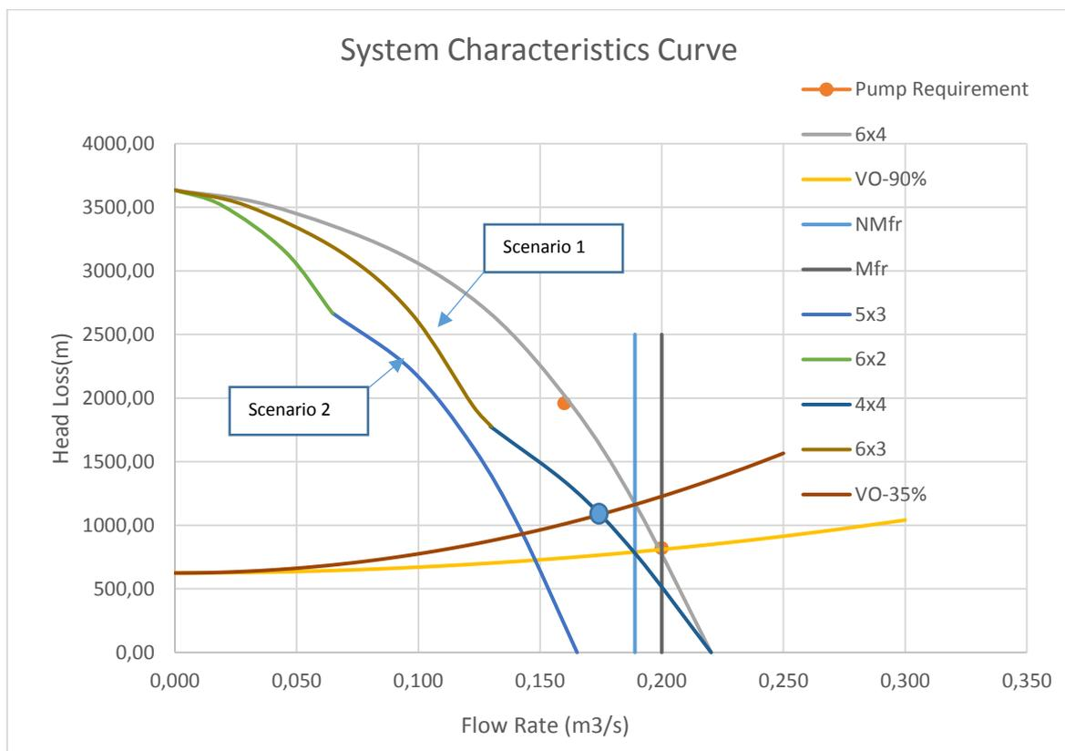
Figure 3.2: Pump Station 1 with 2 Pump failed
