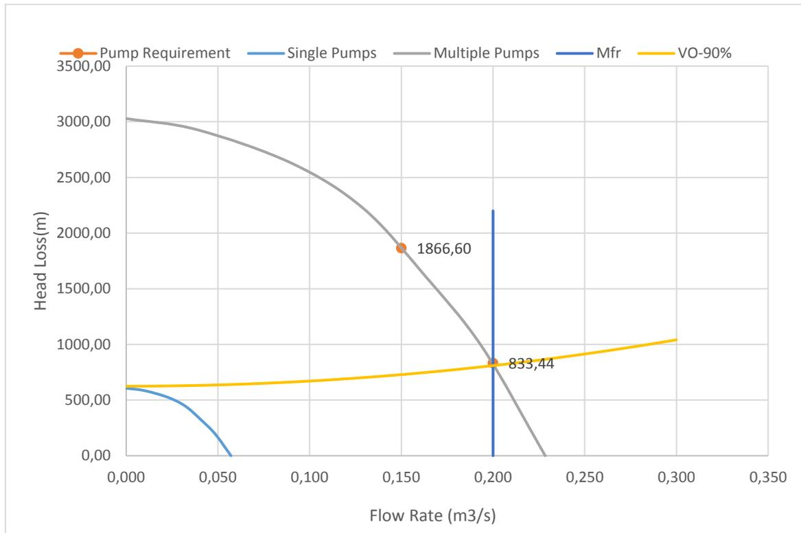
Figure 2.12: Characteristic Curve for Pump Station 1 (Scenario 2) at 90% Opening
