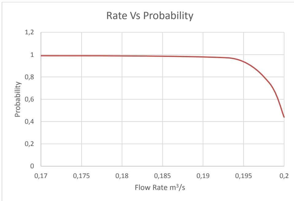
Figure 3.9: The probability of achieving a range of flow rates after failure for pump station 3
