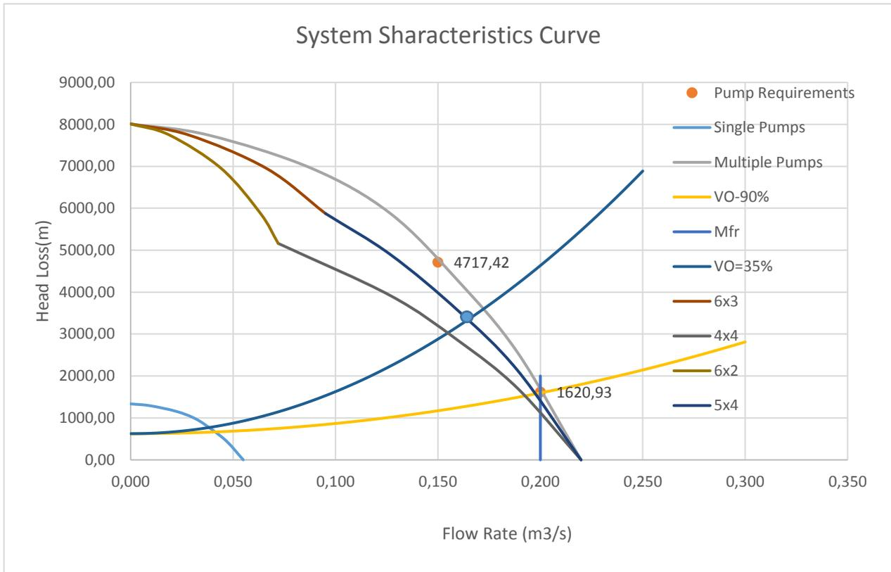
Figure 3.17: Pump Station 2 with 2 Pumps failed
