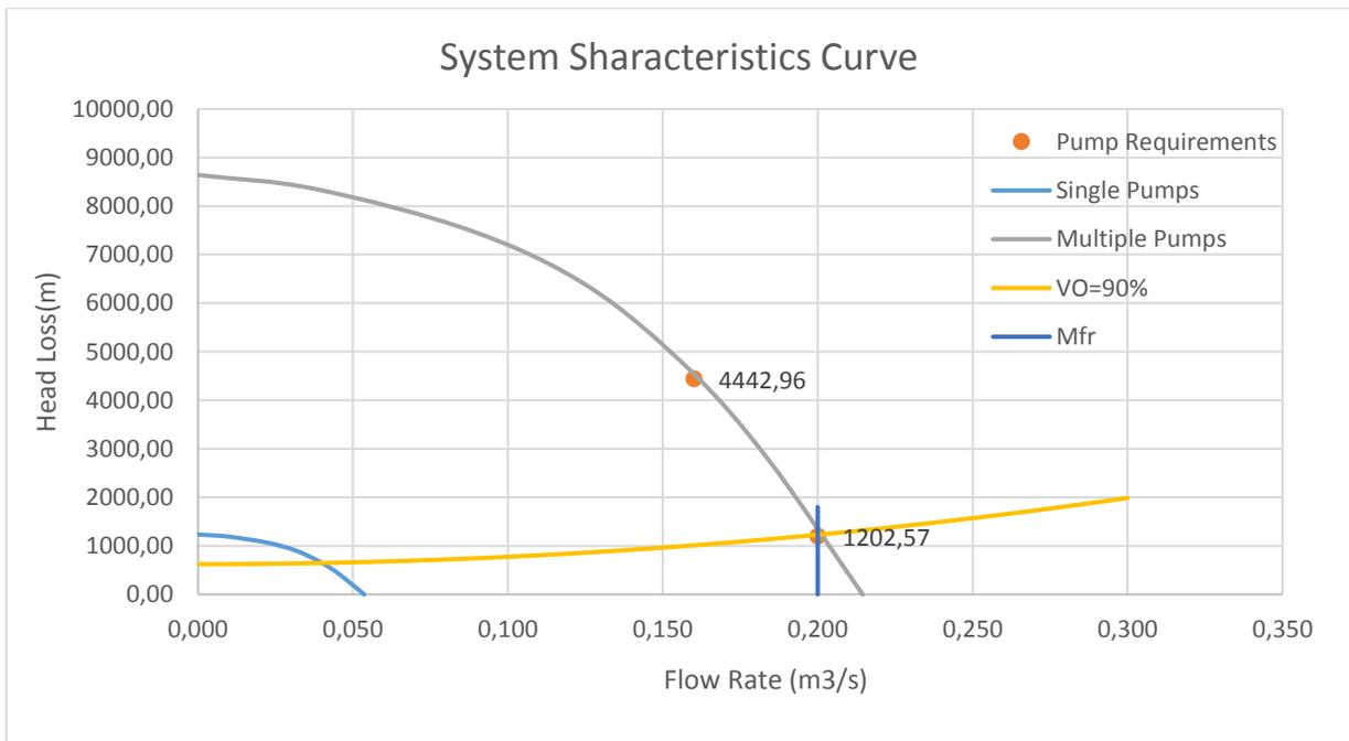
Figure 2.8: Characteristic Curve for Pump Station 4 at 90% Opening
