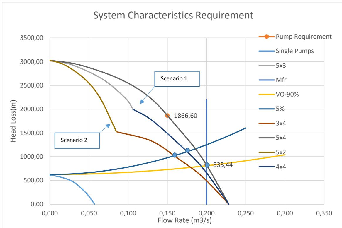
Figure 3.14: Pump Station 1 with 2 Pump failed
