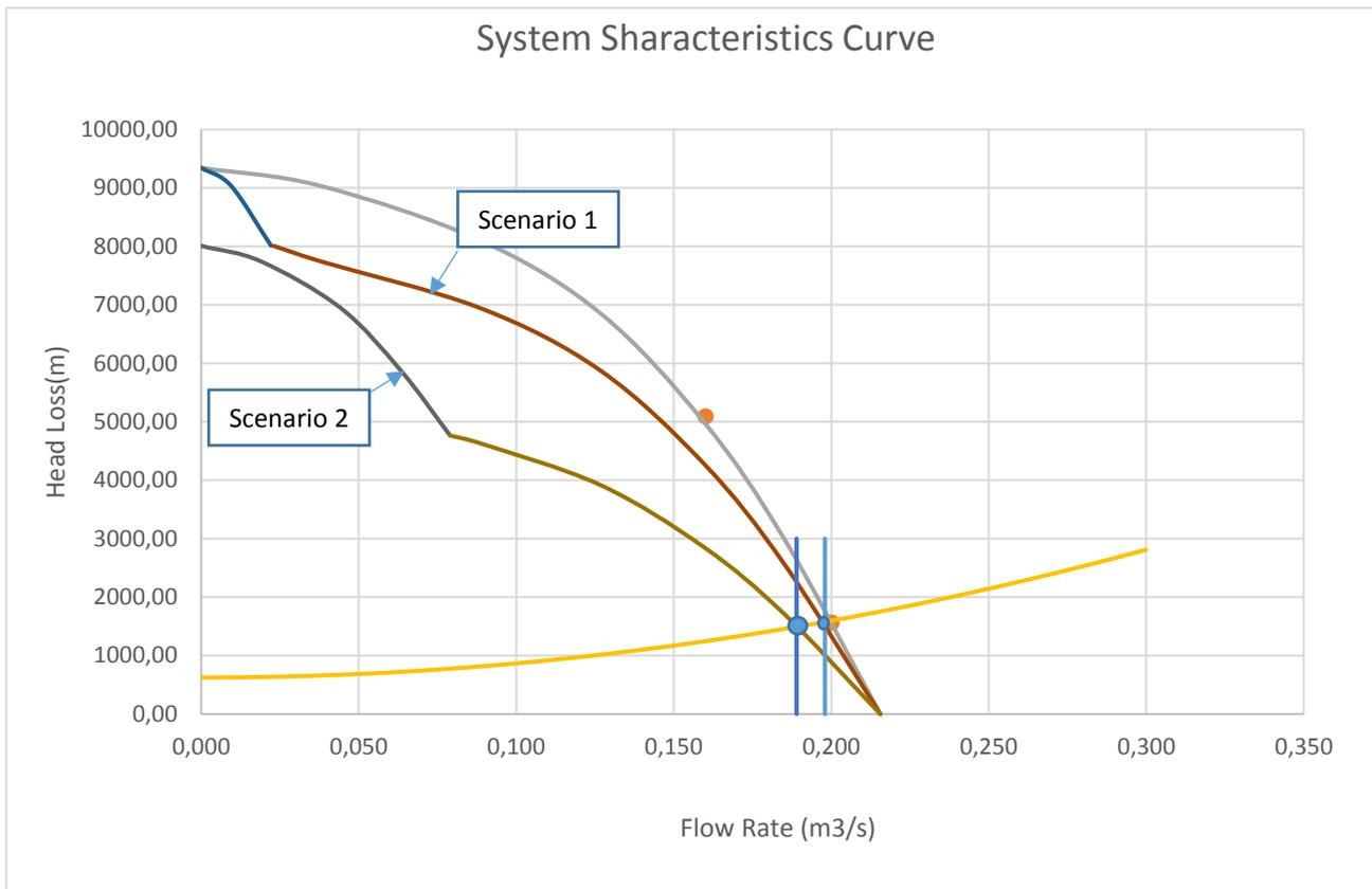
Figure 3.18: Pump Station 2 with 3 Pumps failed
