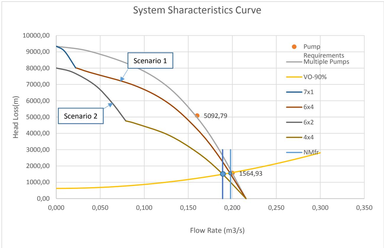
Figure 3.6: Pump Station 2 with 3 Pumps failed
