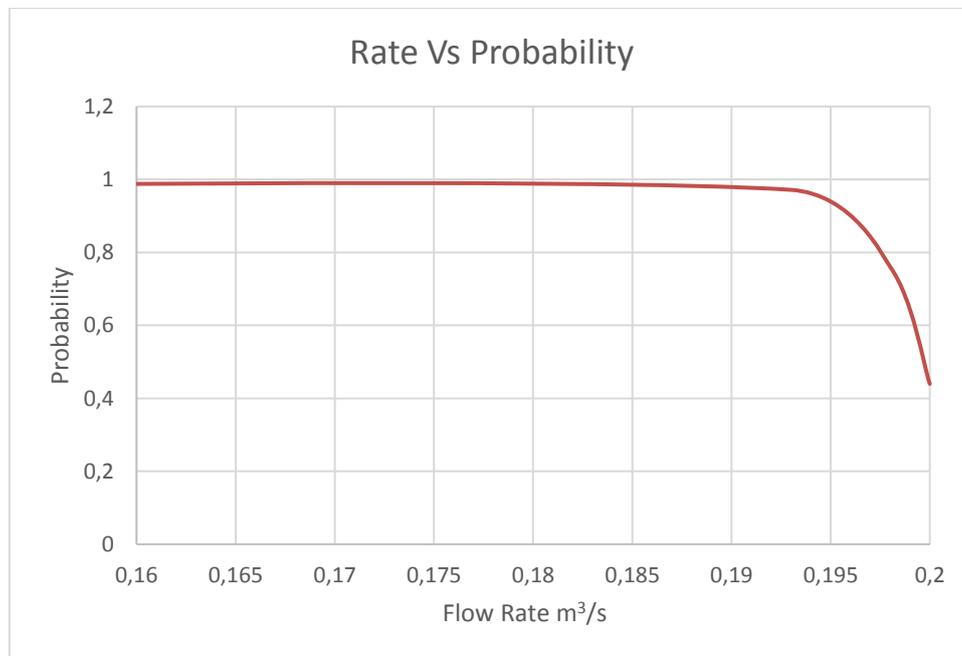
Figure 3.20: The probability of achieving a range of flow rates after failure for pump station 2
