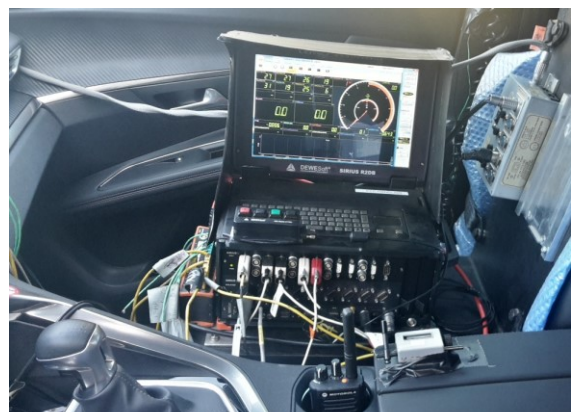
Figure 30. Data Acquisition System mounted instead of the front passenger seat.
