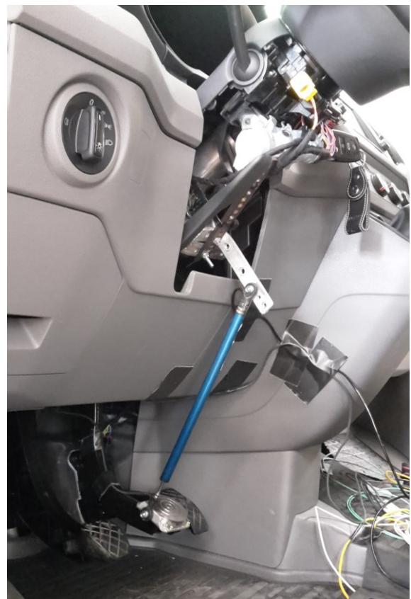
Figure 26. Brake pedal travel sensor (blue) and pedal force transducer (circular pad on the brake pedal).
