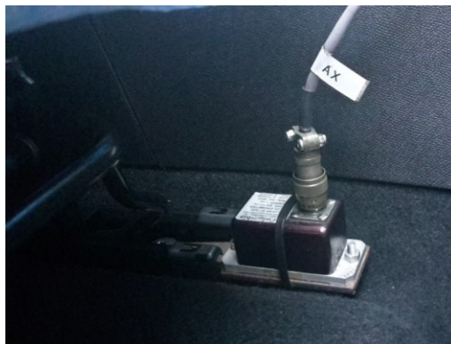
Figure 28. Longitudinal acceleration sensor mounted on the fixed part of the front seat slide.
