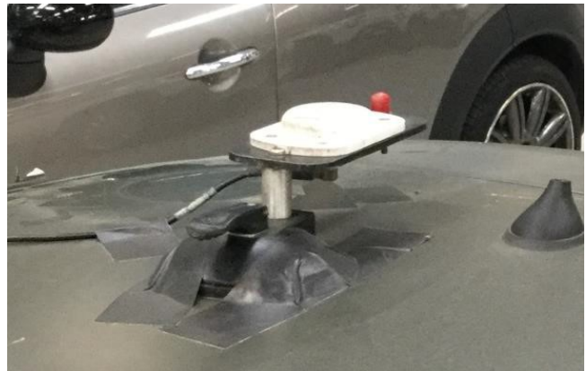
Figure 27. Roof-mounted GPS antenna and its metallic support.
