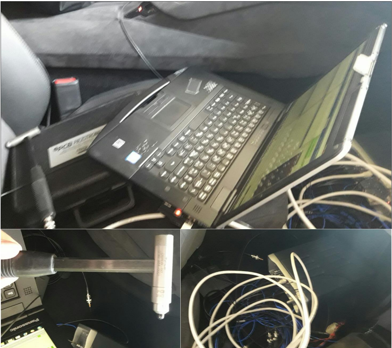
Figure 2.47: instrumentation for the data acquisition of the impact test
