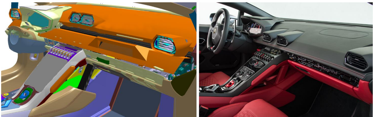
Figure 3.1: DMU rendering of the dashboard with the remodelled CCB (on the left) compared with the current Huracán dashboard (on the right)
