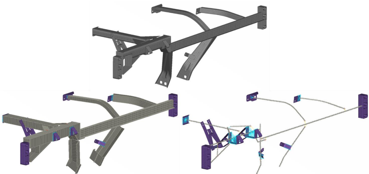
Figure 3.15: comparison between the models of the current CCB with 2D elements, on the top, and 1D elements, on the right bottom. On the left the 1D model is represented with the cross-sections of each beam displayed
