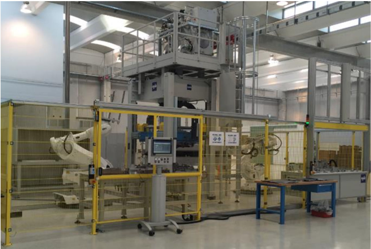
Figure 2.29: automated thermoform line used for the production of the components in thermoplastic CFRP laminates
