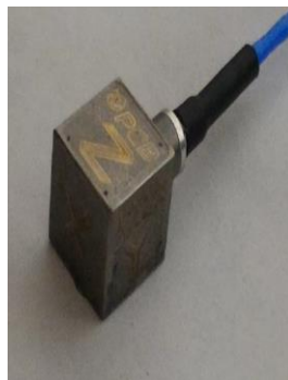
Figure 3-6: Accelerometers PCB TLB356A12 and their specifications
