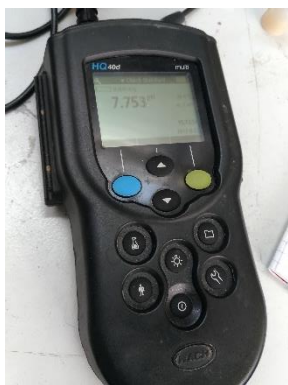
Figure 35 HQ40d Portable multimeter: pH, conductivity and dissolved oxygen for water
