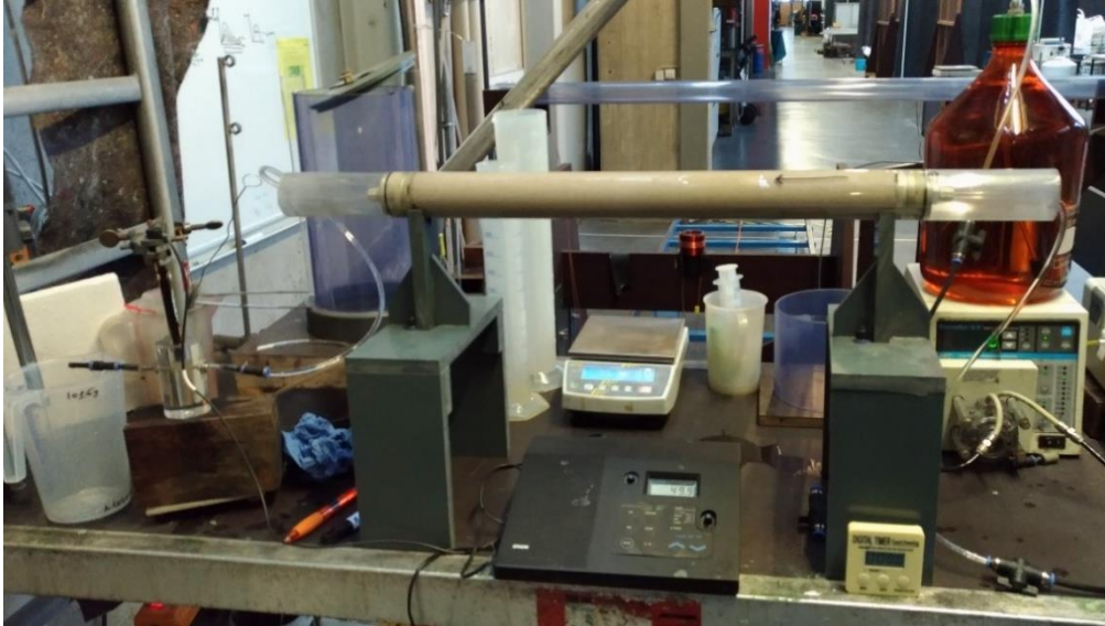
Figure 53 Experimental setup for tracer tests. From right to left: degassed water tank, peristaltic pump, sand-packed column and flow cell with bromide sensor
