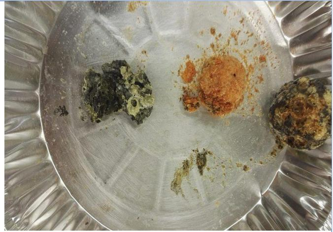
Figure 49 Mobile phones after heated aqua regia digestion
