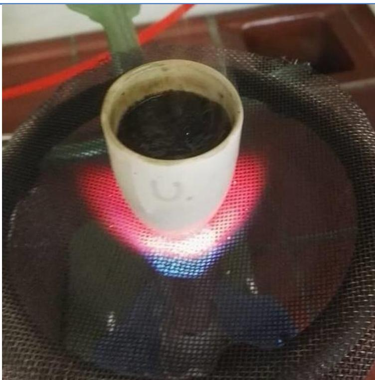
Figure 41 Laptop preburning, during the increase of volume
