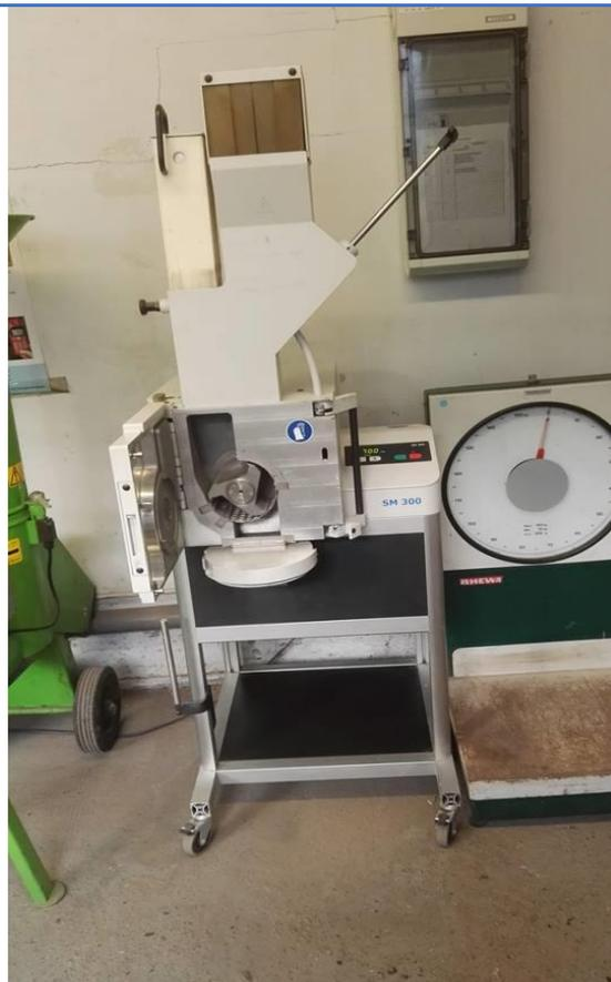
Figure 17 Blade crusher
