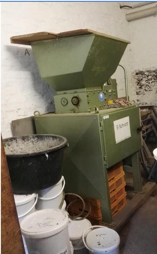
Figure 16 Blade shredder
