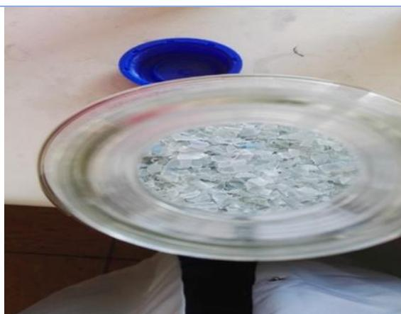
Figure 27 Shredded and washed PET
