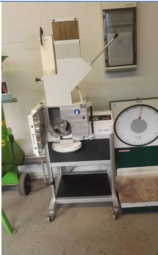
Figure 17 Blade crusher
