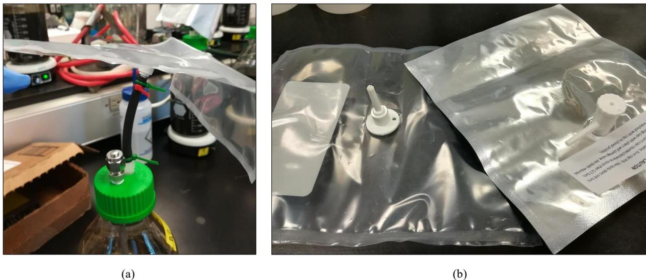
**Figure 3.5:** System for the collection of biogas: (a) A neoprene tube, closed by means of plastic ties, connects the headspace of the reactor to the gas bag; (b) on the left the first gas bag equipped with a push lock valve, on the right the second gas bag with a screw cap valve.
