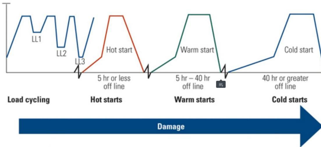
**Figure 9 - Relative damage caused by cycling steam plants**
