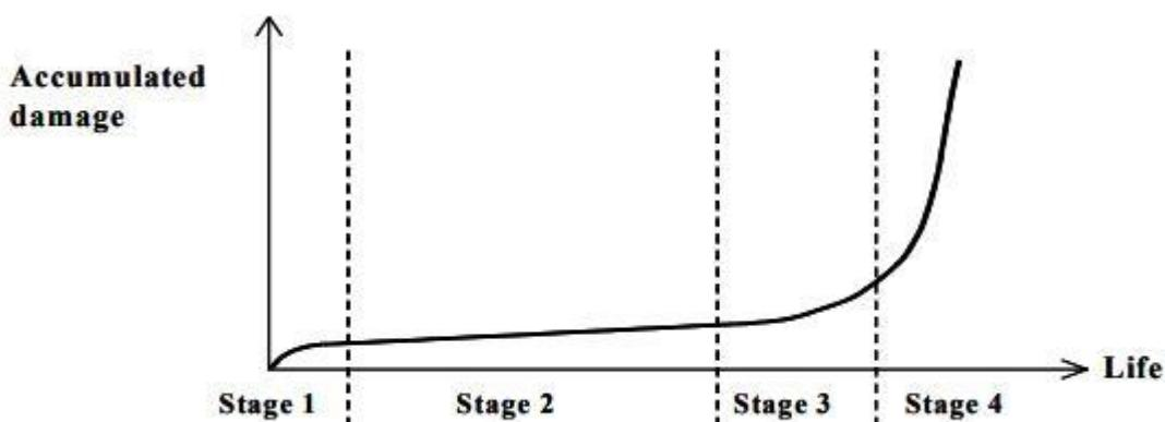
**Figure 5 - Variation of accumulated damage during equipment service**
