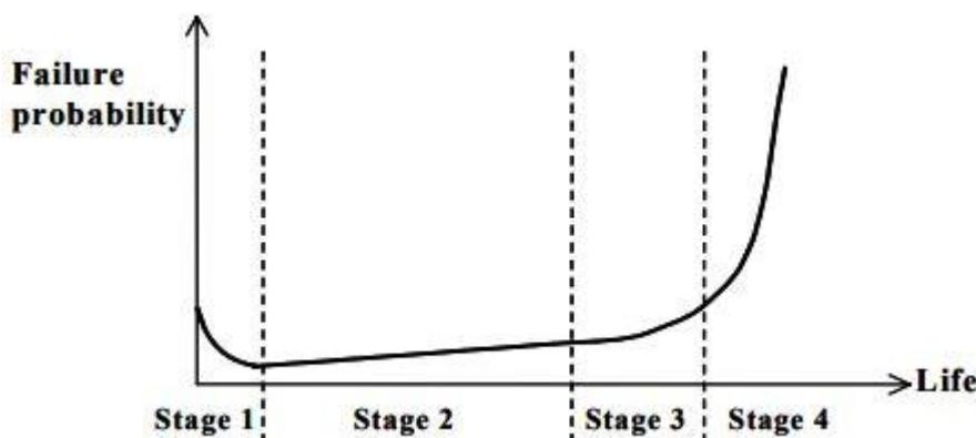
**Figure 7** - Model for the probability of failure of a population of equipment
