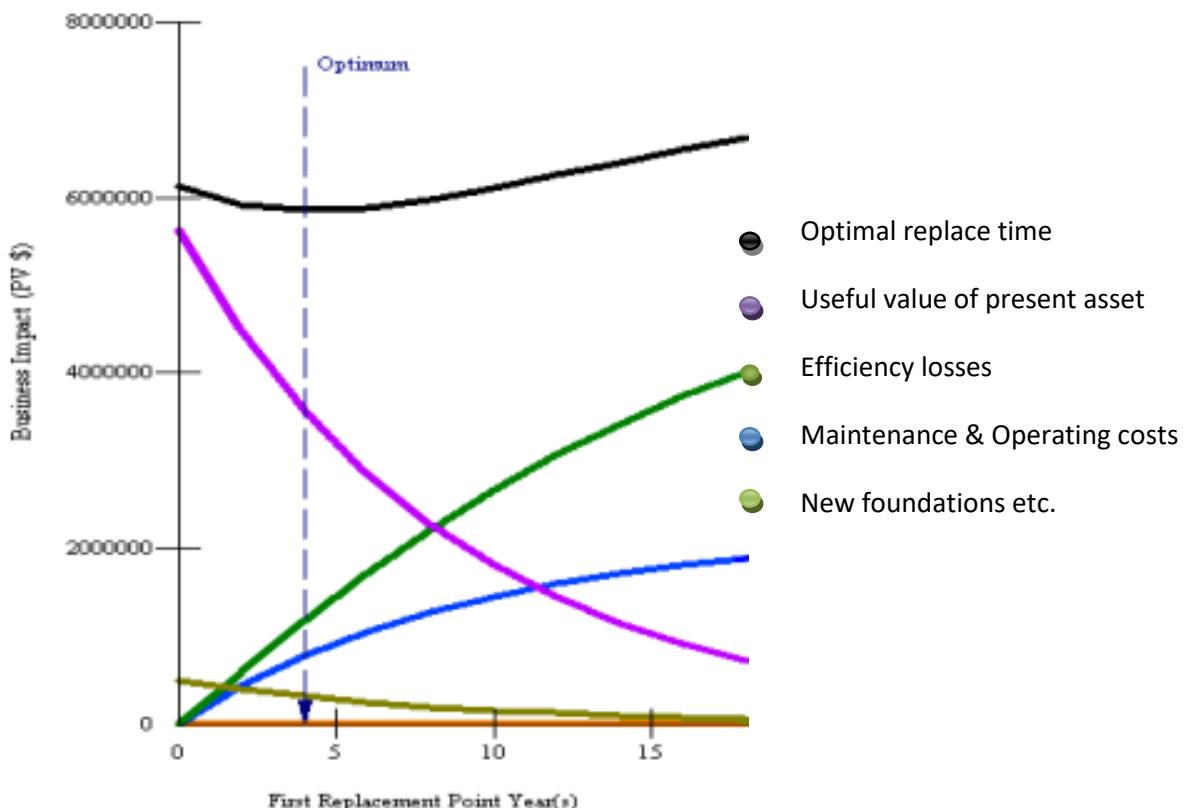
**Figure 14 -** The optimal replacement time of the old existing asset
