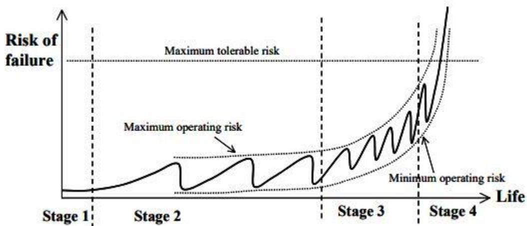
**Figure 6** - Effect of periodic maintenance, inspection and repair on the risk of failure for a piece of equipment, each saw-tooth represents an inspection being carried out
