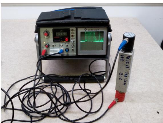
Fig. 32 - Provino 40mm x 40mm x 160mm
