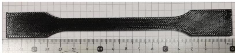
Figura 4.1 Provino A1 (XY)
