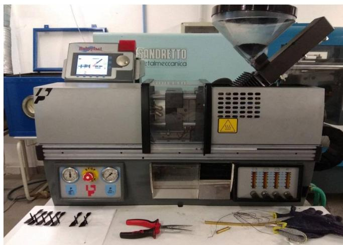
**Figure 3.5** - Babyplast injection molding machine, 6/10P model, manufacturered by Cronoplast S.L.
