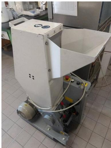
**Figure 3.4** - Pelletizing machine Piovan, RSP 15/15 model.
