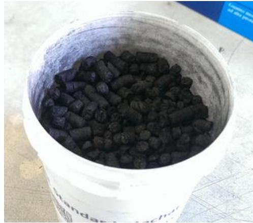
**Figure 2.3** - Biochar pellets derived from oil seed rape straw.
