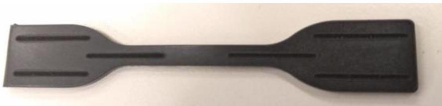
**Figure 3.11** - The experimental layout for a generic sample: three laser tracks per trial, two trials per sample.
