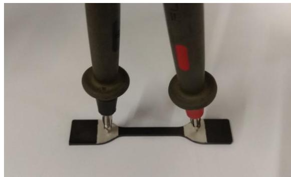
Figure 3.7 - Linear surface resistance measurements per unit length on non-lasered specimens. The multimeter tips are placed directly on the two electrodes.
