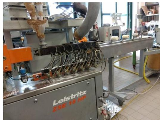
**Figure 3.3 - Twin screw extruder Leistritz ZSE 18 HP-PH.**
