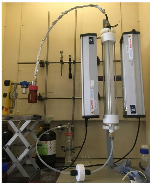
Figure 2.16: Complete equipment: atomizer, photo-reactor, filter.
