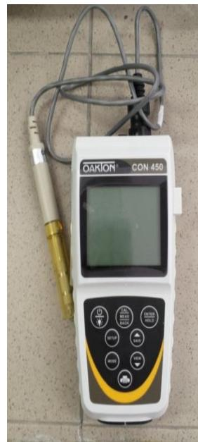
Figure 12. Conductimeter used.
