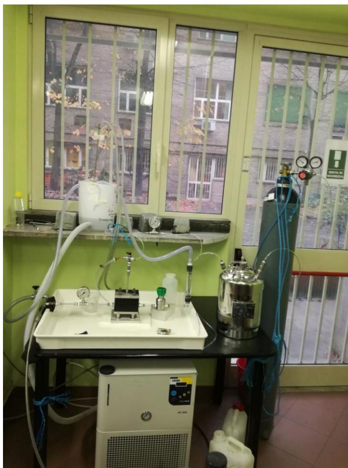
Figure 10. Backwashing System with Crossflow.
