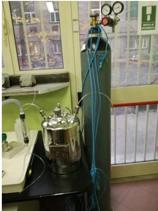
Figure 11. Tank with DI water and Nitrogen Vessel.
