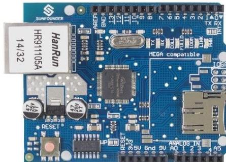
Figura 26 - Ethernet Shield
