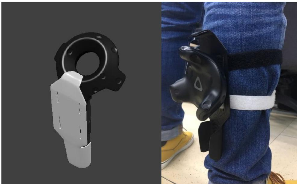
Figura 5.18: Rendering of the support for the leg Controller on the left, Support adapted to work with Tracker on the right
