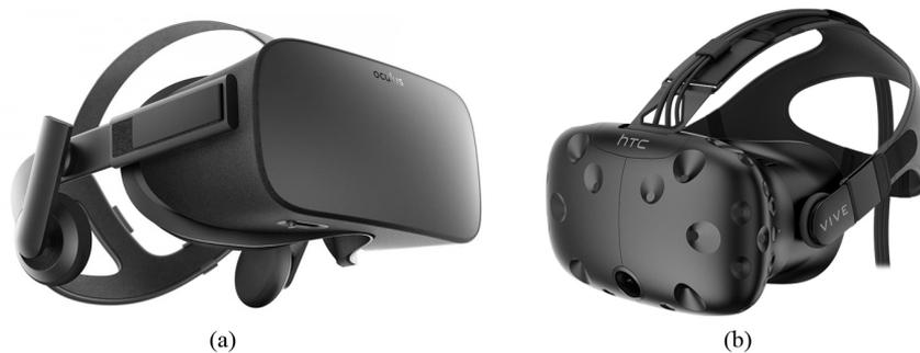
Figura 1.3: Oculus Rift CV1 (a), HTC VIVE (b).
