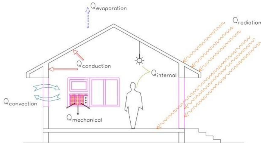
Figure 3.5 – Heat exchange processes between a building and the external environment
