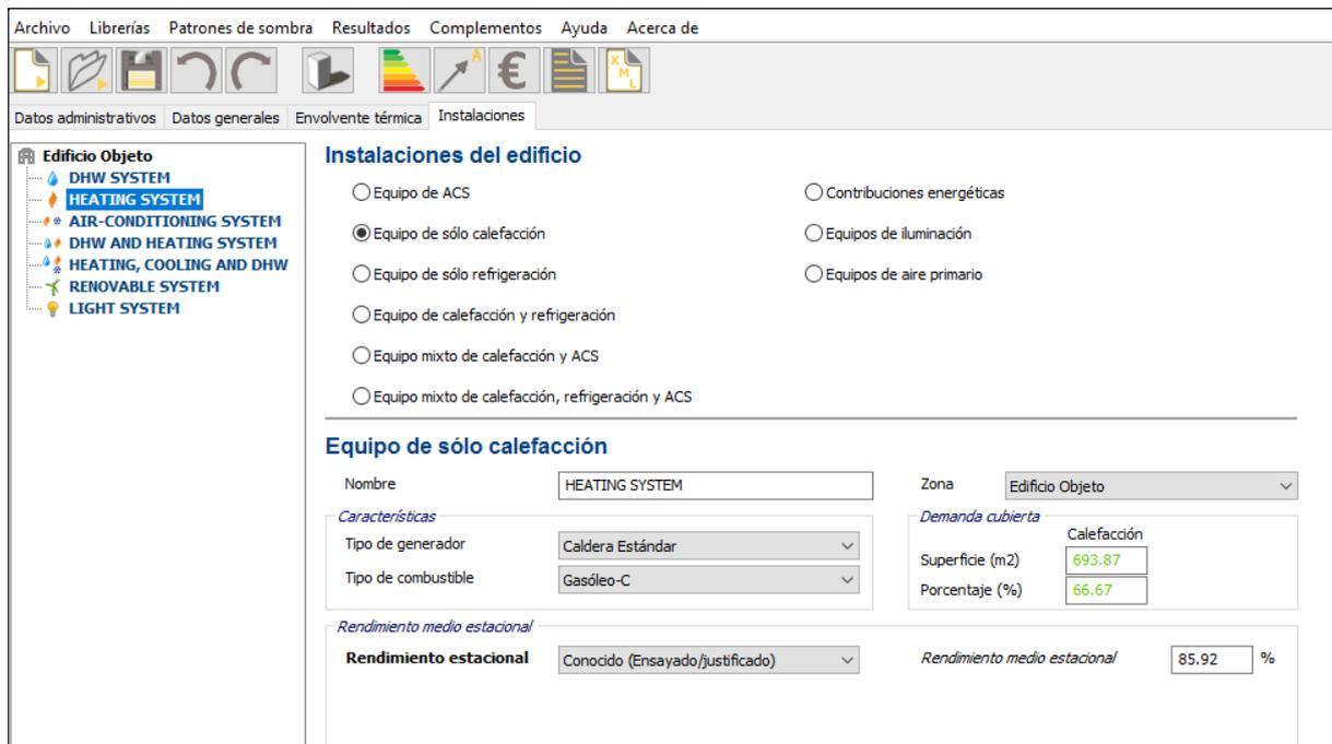
Figure 6.31 – Insertion of heating system. CE3X Screenshot
