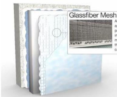
The glassfiber mash is applied to the insulation panel to reinforce its impact resistance. The mesh is embedded in the base coat.
