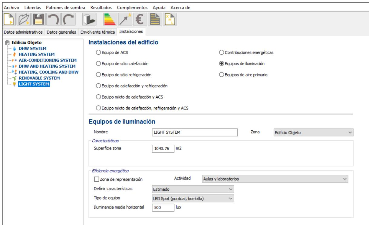
Figure 6.32 – Insertion of light system. CE3X Screenshot
