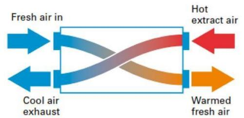
Figure 4.11 – Illustration of heat recover
