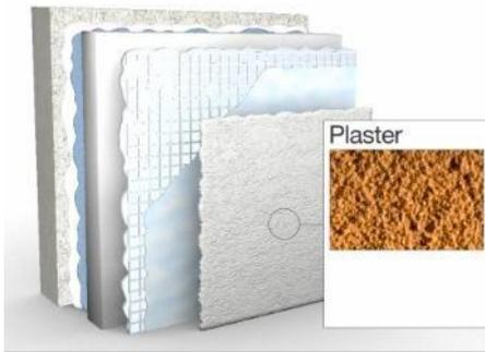
Typical coating include hydrophobic plasters made of mineral, acrylic, silicate or silicone. is one of the least expensive and most often used facade materials for new buildings and renovation projects in Europe.
