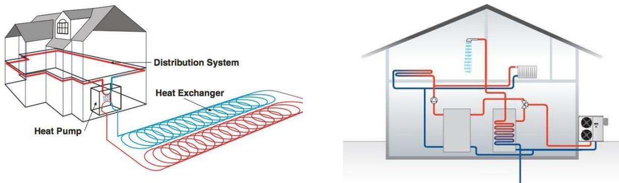
Figure 4.3 – Ground-source heat pump (left); Air-source heat pump (right).
