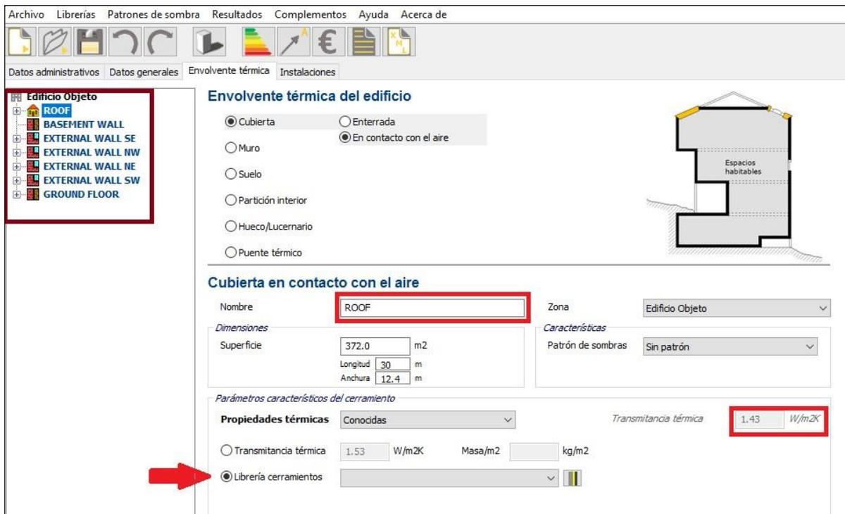
Figure 6.23 – Insertion of roof. CE3X Screenshot
