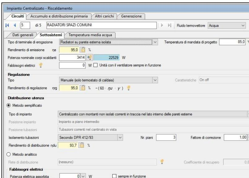
6.65 – Subsystems of heating system
