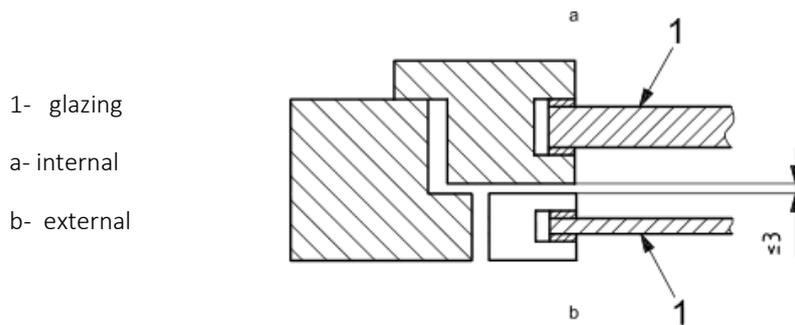
Figure 3.12 – illustration of coupled windows
