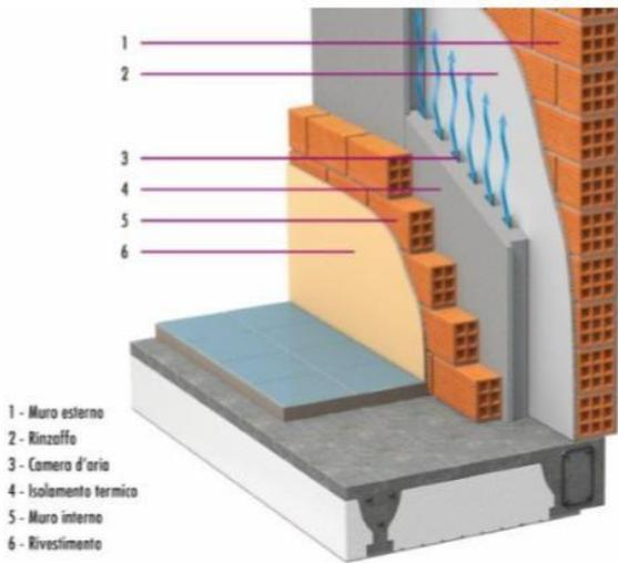
Figure 3.27 – Façade with Middle Insulation
