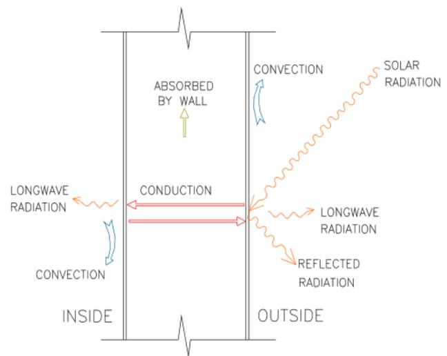
Figure 3.7 – Heat transfer processes occurring in a wall.
