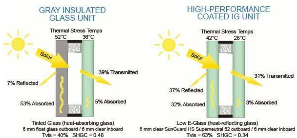
Figure 3.16 – Glazing insulation performance
