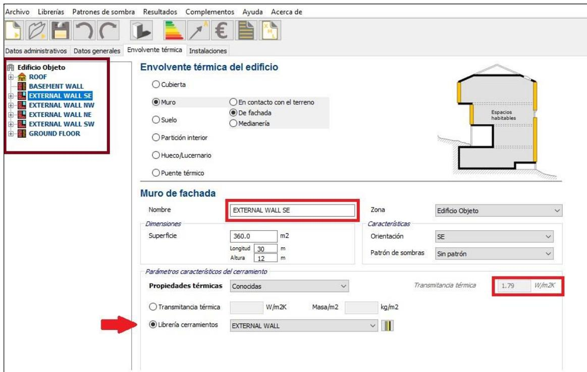
Figure 6.25 – Insertion of external wall. CE3X Screenshot
