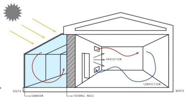
Figure 3.4 – Isolated gain passive solar Energy.
