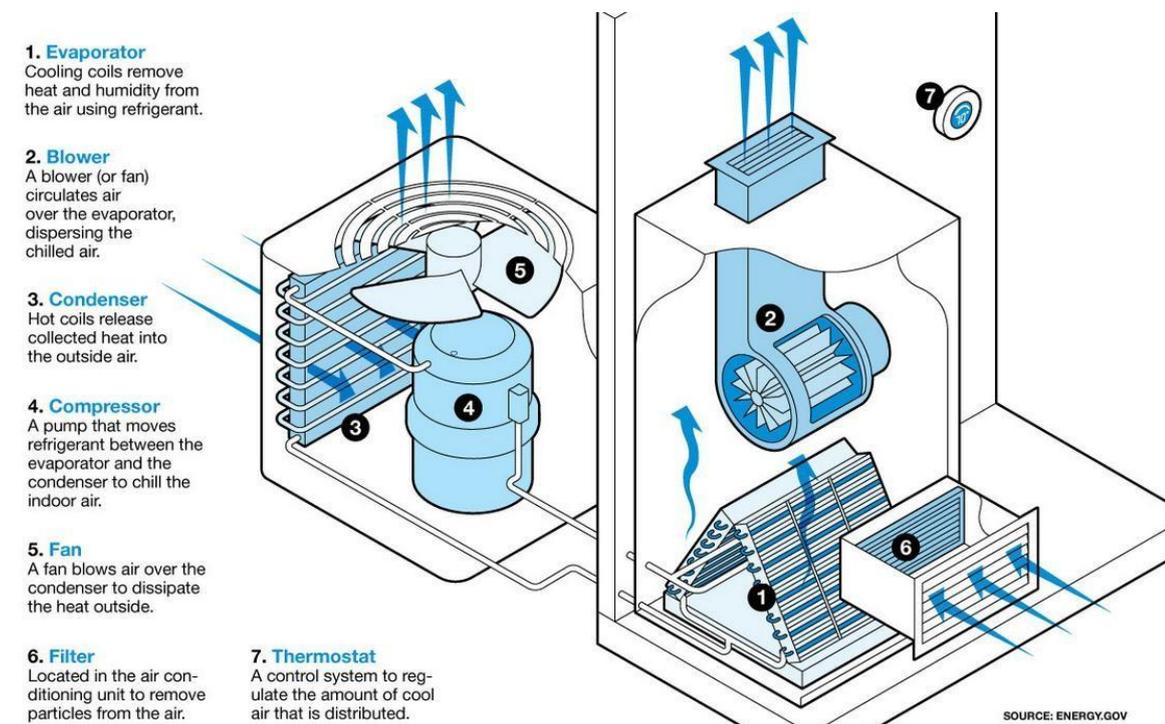
Figure 4.8 – Illustration of how an air conditioner work.
