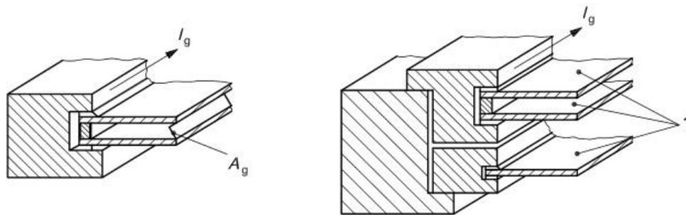
Figure 3.9 - illustration of glazed area and perimeter
