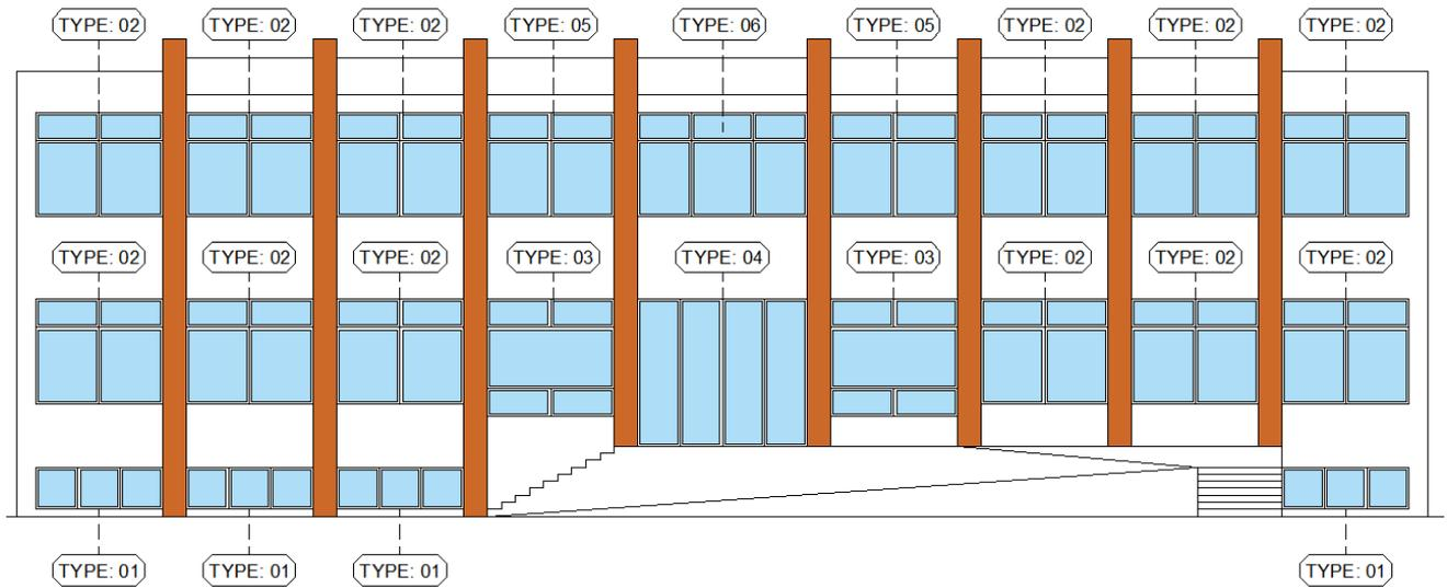
Figure 6.13 – Scheme of type of windows. South-East façade
