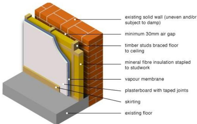
Figure 3.26 – Façade with Internal Insulation
