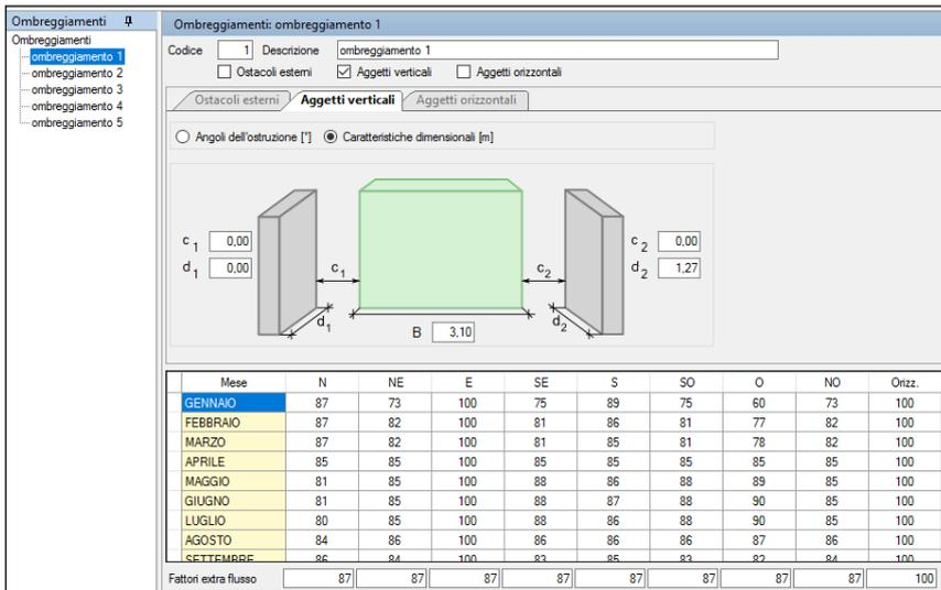
When the buildings component are all defined, their shadows will be introduced. The building has vertical bosses that will be inserted in the program. The dimension of bosses and the distance between them will be put. The building has 5 types of shading.
