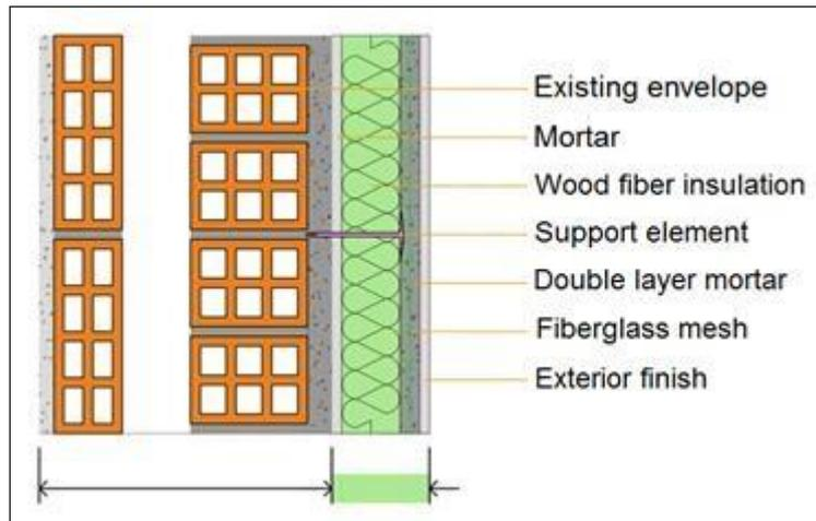
Figure 6.39 – New façade with ETICS solution
