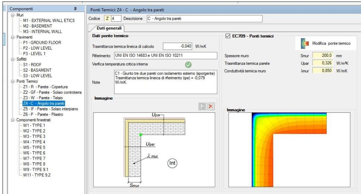
6.57 – Thermal bridge of corner between walls
