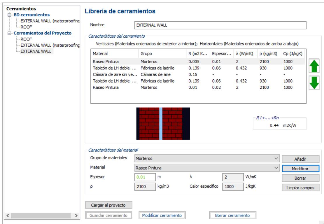
Figure 6.26 – Insertion of external wall details. CE3X Screenshot
