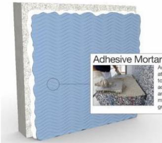
Adhesive mortar is used to attach the insulation system to the exterior wall.
