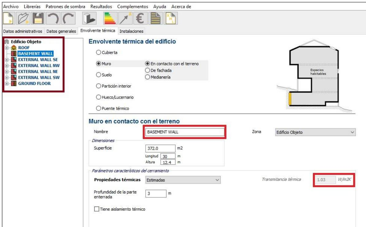
Figure 6.22 – Insertion of basement wall. CE3X Screenshot
