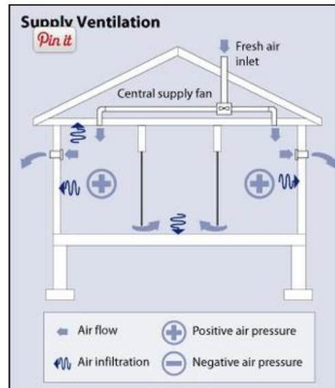
Figure 4.10 – Illustration of supply ventilation system.
