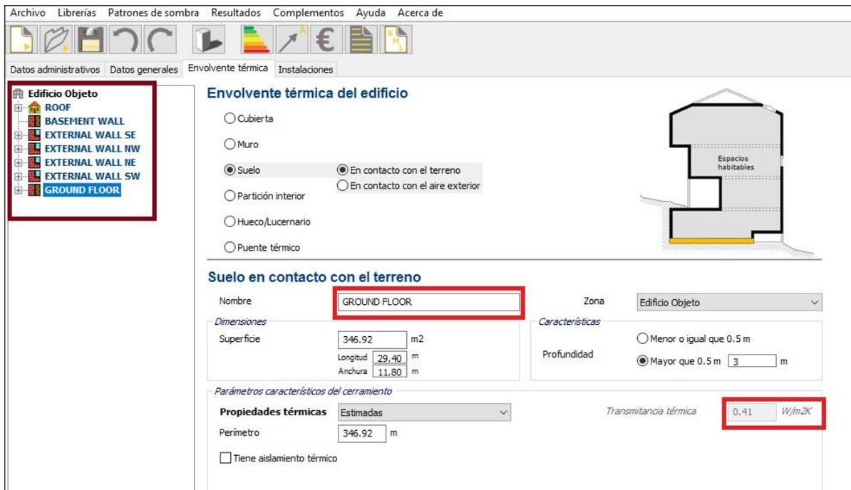
Figure 6.21 – Insertion of ground floor. CE3X Screenshot
