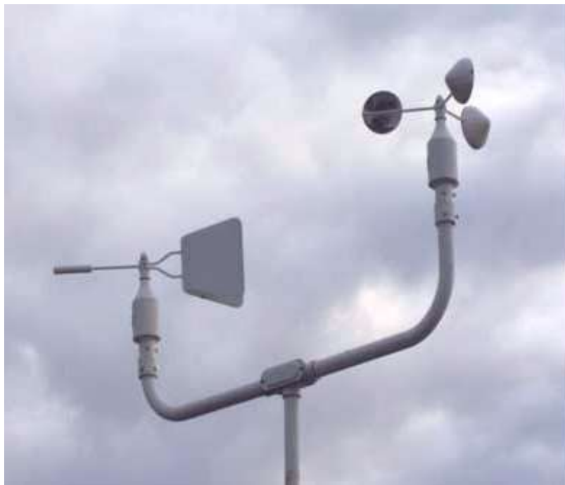
Figure 34: A wind vane and rotating cup anemometer. Source: http://learningweather.psu.edu/node/10 consulted on 30/06/2017.
