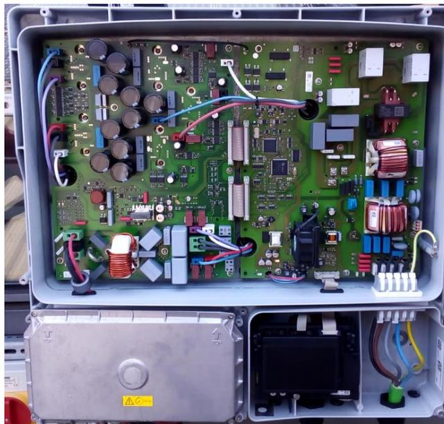
Fig.5.1 Interno inverter
