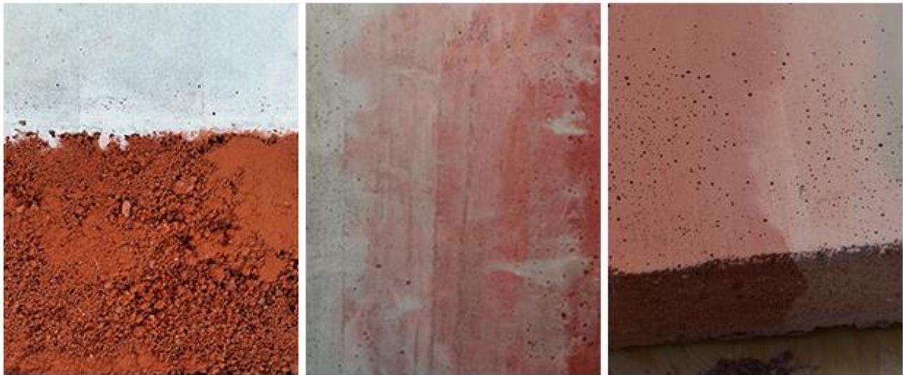
Figure 2: Concrete test with insertion of red soil into the mixture (Red Soil)
