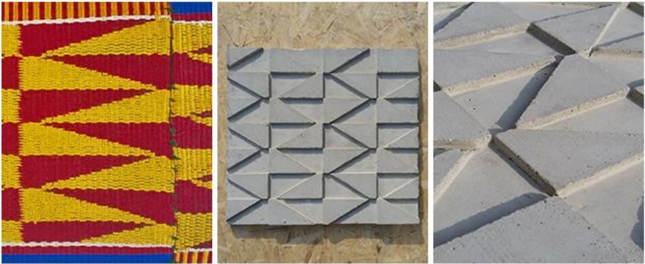
Figure 1: Concrete test with the study of Kente pattern (Kente in formwork)
