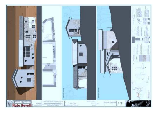
It is a semi-hypogeal building with the same layout as the other buildings of the village, which combines, in a simple way, three blocks as in the spontaneous alpine architecture. The simple clear lines of the new building are made to match the old ones, highlighting the distance between the old and the new, but at the same time starting a dialogue between them.
