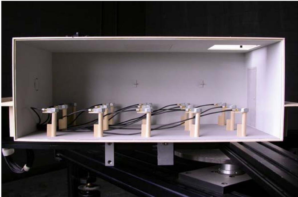
I have analysed different typologies of pipes, varying: the finishing materials (specular films, white diffusing painting and OLF microplasmatic films); the pipe length, up to 9 metres (about 10 yards); the section shape, circular or square; the pipe position with respect to the environment, central and eccentric. The patterns have been subjected to several sky conditions at different times of the year and day.
