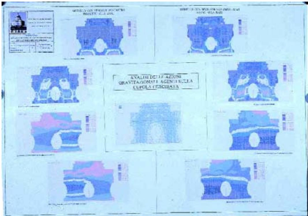
Each single arch generally presents a situation of press-flexion at the impost hewn stone, with tension of traction at the intrados and of compression at the extrados. Vice versa, at the reins the situation is the other way around, with solicitations of traction toward the outside and of compression toward the inside.
