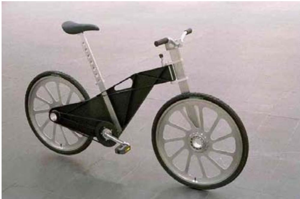
An outstanding feature is that most of the mechanical functions, such as freewheel, coaster brake and possibly the gears, can be concentrated in a sealed shell located in the bottom bracket area, so that all the bike can be left neat and simple. The rear wheel for example can be detached without any operation on the drivetrain, thanks to the mono-arm structure, while not a single cable-housing combination is used.
