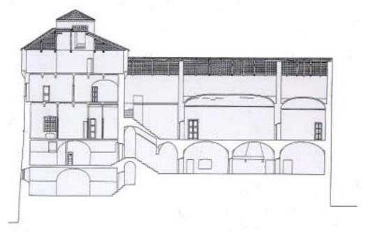
With the help of graphic and analitical methodologies, I have verified the stability of the barrel valuts and of the cross vaults located in the 17<sup>th</sup> century section of the castle.
