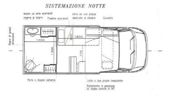
The graduation thesis provides 3 plans in order to give different solutions 3 plans in order to give different solutions of accessibility to the motor-home bound for disabled persons.
