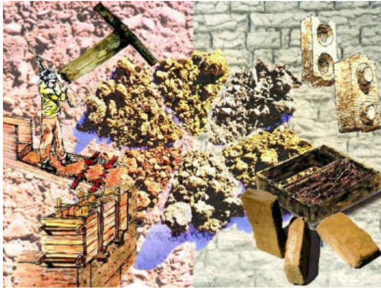
Picture 1 - Building typologies that can be compared with each other: the rammed earth (left) and the adobe (right). The rammed earth was obtained by pressing the clayey soil in a wooden mould with a particular beating instrument. Furthermore, the buildings were toothed with some crowns in locust-tree wood. On the contrary, the green bricks were realised with a list of wood, by means of sifting soil; when they were dry, they were finally employed. Fluid ground was used like a cementing substance. The theme of the adobe was provided by Professor Roberto Mattone who patented a stabilised block. This block was obtained thanks to a hand press.
