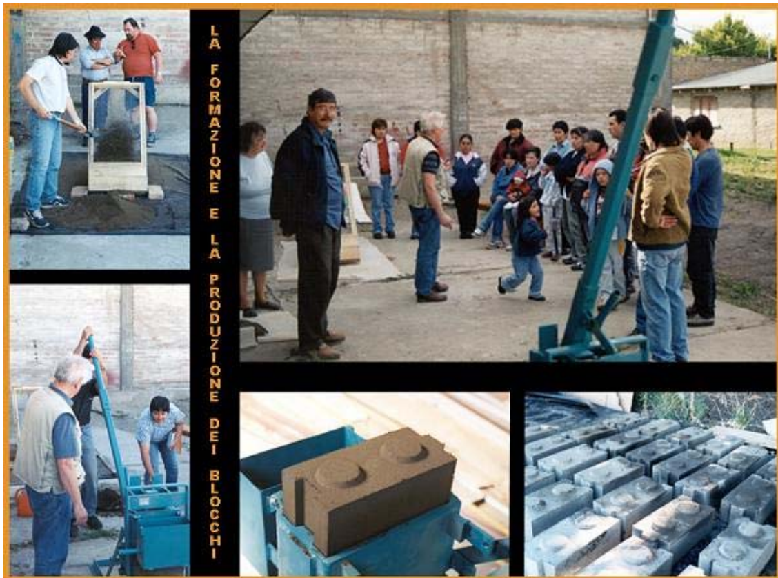
Picture2: the training course and the manufacturing of blocks of earth shaped like “bricks”
