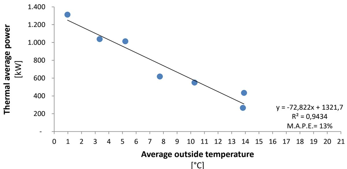
The Figure 1 shows an example of energy signature and in particular the strong linear relationship between consumption and temperature also for analysis at monthly scale.
