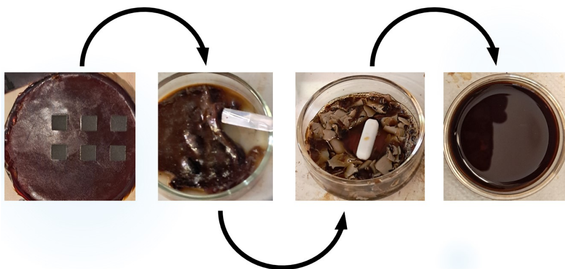
Figure 3.10: Recycle process of the porcine gelatin substrate from the final LIG product to the regenerated liquid state.
