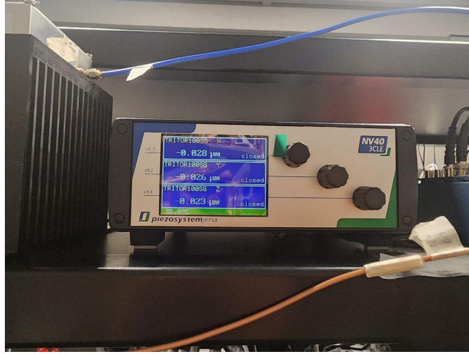
Figure 3.10: Piezoelectric stage controller used for precise three-dimensional positioning of the diamond sample during confocal scanning.
