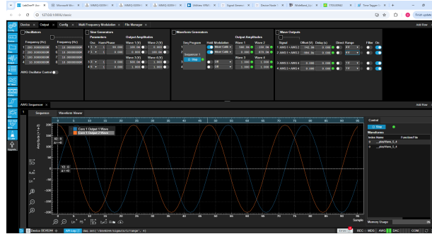
Figure 5.5: LabOne interface used during the calibration of the HDAWG and the AM0350A IQ mixer. The upper panels provide access to the oscillator configuration, waveform generation, output amplitudes, DC offsets and voltage ranges of the analog channels, while the waveform viewer at the bottom displays the synchronized I and Q baseband signals before frequency up-conversion. These controls were used to iteratively optimize the IQ mixer calibration by minimizing the local oscillator leakage and the unwanted image sideband observed on the spectrum analyser.
