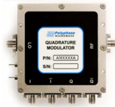
Figure 5.2: Polyphase Microwave AM0350A quadrature modulator used as the external IQ mixer in the up-conversion chain. The device converts baseband I/Q signals to an RF output and is specified for operation from 300 MHz to 5000 MHz. Figure adapted from the manufacturer’s datasheet [25].
