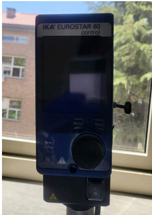
Figure 4.2 — IKA EUROSTAR 60 control overhead stirrer (IKA-Werke GmbH, Staufen, Germany) used for mechanical mixing of the mortar batches.
