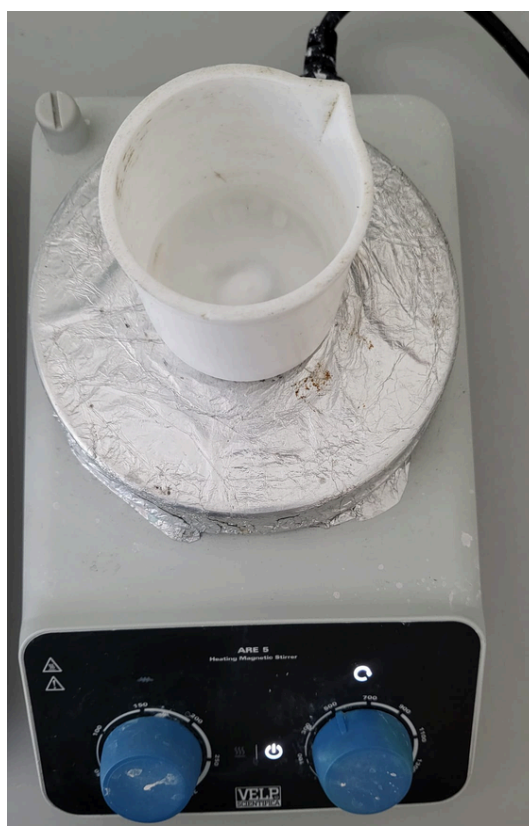
Figure 4.1 — Preparation of the alkaline activator on a VELP Scientifica ARE 5 magnetic stirrer (stirring only, no applied heat), with the sodium silicate–NaOH solution in a plastic beaker.
