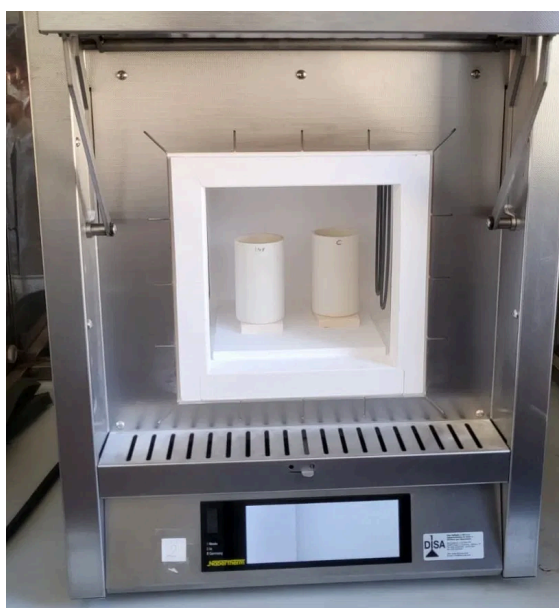
Figure 3.4 — Nabertherm muffle furnace loaded with ceramic crucibles containing sediment fractions prior to calcination at 700°C (programme P16 CALCINATION-700), Politecnico di Torino.
