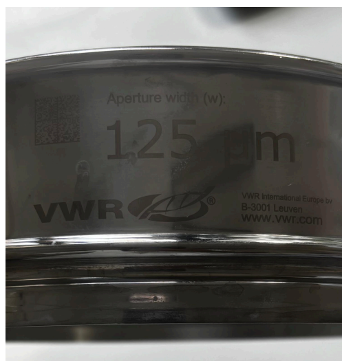
Figure 3.3 — Stacked test sieves (CDL, ISO 3310-1) used for particle separation; the 125 \mu\text{m} sieve shown was applied to the heated series prior to calcination, following the 500 \mu\text{m} primary sieving.
