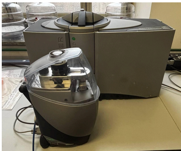
Figure 3.7 — Malvern Mastersizer 3000E laser diffraction analyser with Aero S dry dispersion unit, Politecnico di Torino.
