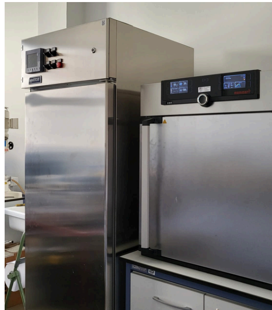
Figure 4.4 — Memmert convection oven (right) used for curing at 60 °C, alongside the laboratory cabinet (left); the display shows the 60 °C set-point.
