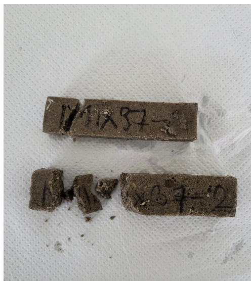
Figure 4.5 — Specimens MIX37-1 (top) and MIX37-2 (bottom) after the 24-hour water immersion. MIX37-1 remained largely intact, whereas MIX37-2 fractured and partially disintegrated during immersion. A leachate-pH reading was still obtained for this mix (Table 5.4), but the damaged specimens were not taken forward to mechanical testing.
