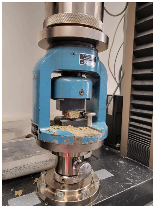
Figure 4.8 — Compressive strength test: a half-specimen (labelled) is crushed between the platens of the RMU compression jig on the Zwick/Roell machine (50 kN load cell), Politecnico di Torino.
