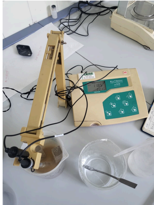
Figure 4.6 — Measurement of immersion-water pH using a Eutech Instruments CyberScan pH 510 meter; with the electrode in the beaker containing a submerged specimen.
