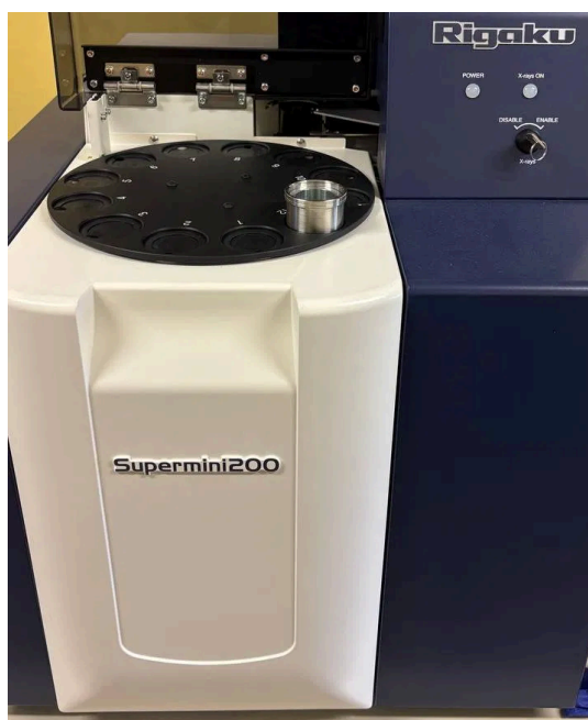
Figure 3.5 — Rigaku Supermini200 wavelength-dispersive XRF spectrometer with the 10-position sample carousel, Politecnico di Torino.
