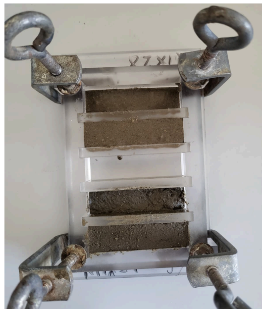
Figure 4.3 — Fresh mortar cast into the prismatic moulds (specimen "MIX 28" shown), compacted by hand and labelled before oven curing.
