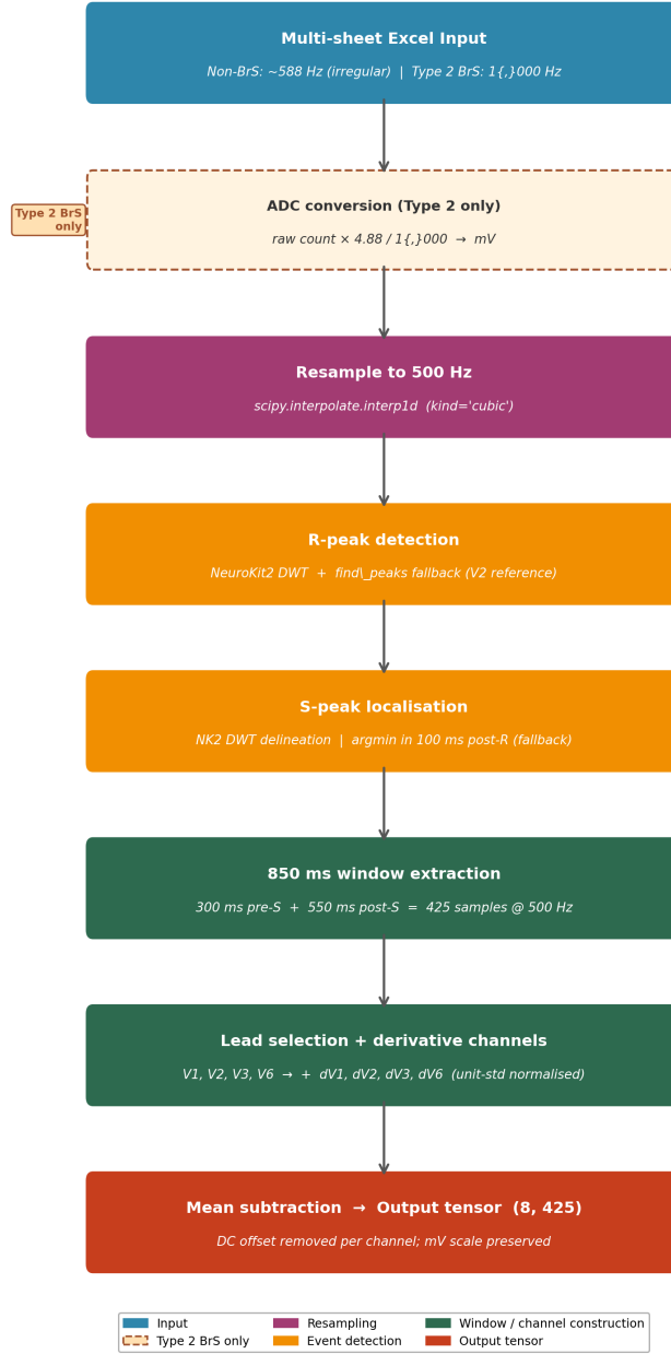
Figure 4.1: Vertical flowchart of the four-stage signal preprocessing pipeline. The ADC conversion step (dashed box) is applied exclusively to Type 2 BrS recordings prior to the shared pipeline. Event detection operates on the V2 reference lead; the resulting S-peak indices are applied uniformly across all four extracted leads (V1, V2, V3, V6). The output tensor shape (8, 425) reflects eight channels (four raw and four derivative leads) at 425 samples per 850 ms window at 500 Hz.
